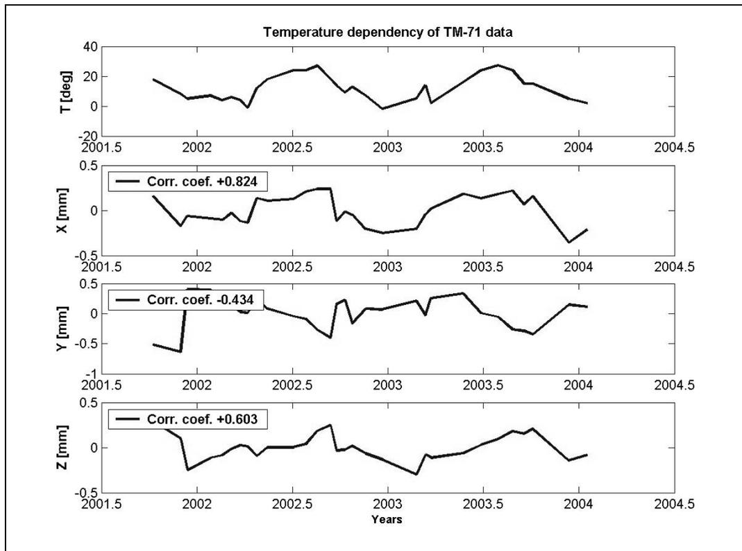
**Fig. 7** Graph of the temperature and displacement time series for the “Dobromierz” TM-71 gauge
