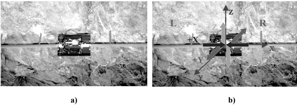
Fig. 2 The TM-71 crack gauge: a) general view, b) orientation of measurement axes
