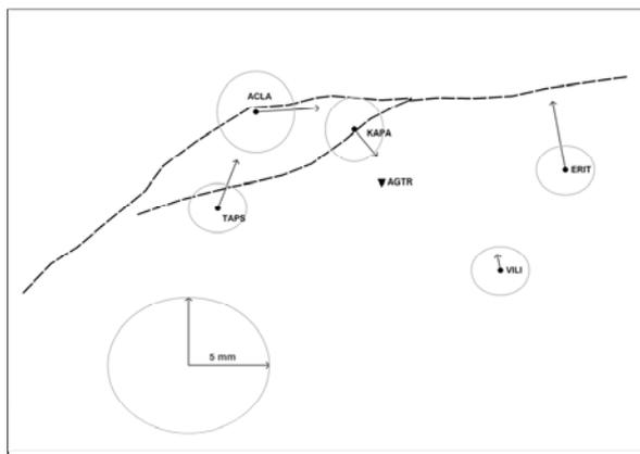
**Fig. 21** Total horizontal displacement vectors of "Kaparelli" network sites.
