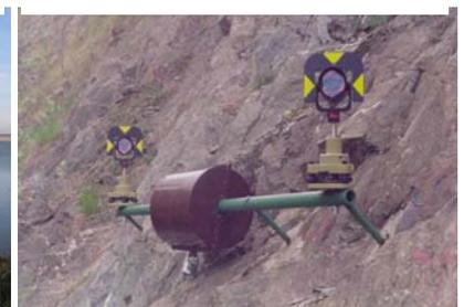
Fig. 9 Crack gauge.
