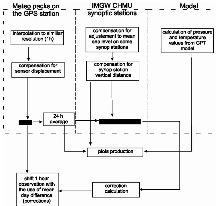
Fig. 2 Data comparison and calibration flow scheme.
