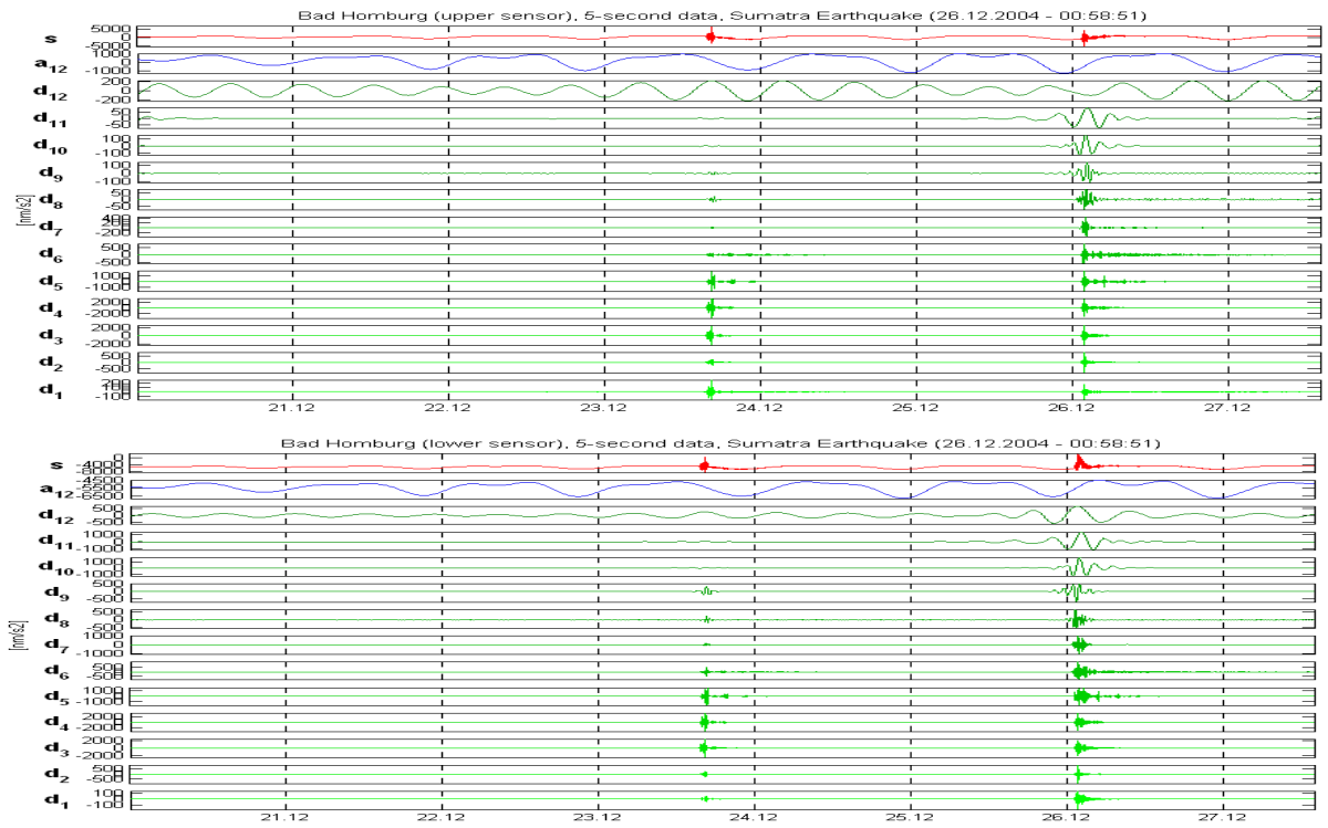
Fig. 5b Wavelet decomposition for the time series from the Bad Homburg station into p=12 frequency components during the Sumatra-Andaman earthquake; top: upper sensor, bottom: lower sensor.
