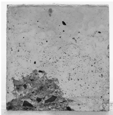
Fig. 3 An example of spalling on the concrete surface (mix-design REC I at temperature 400 °C).
