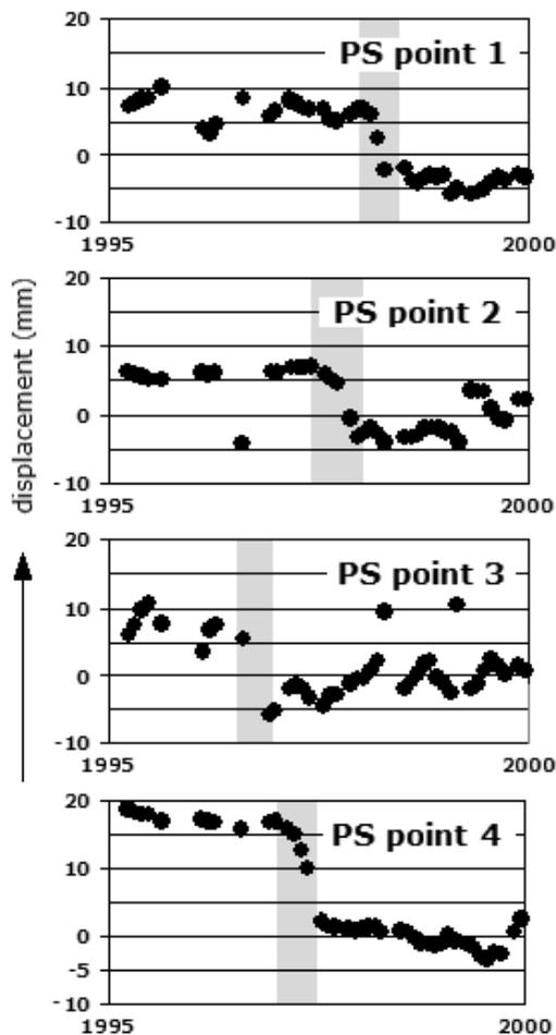
Fig. 4 Time series of displacements of selected PS (marked in Fig. 3) for the 1995-2000 period close to the collection sewer in the Stodůlky locality (the grey column indicates the time interval when the surface displacement for the given scatterer could be observed).
