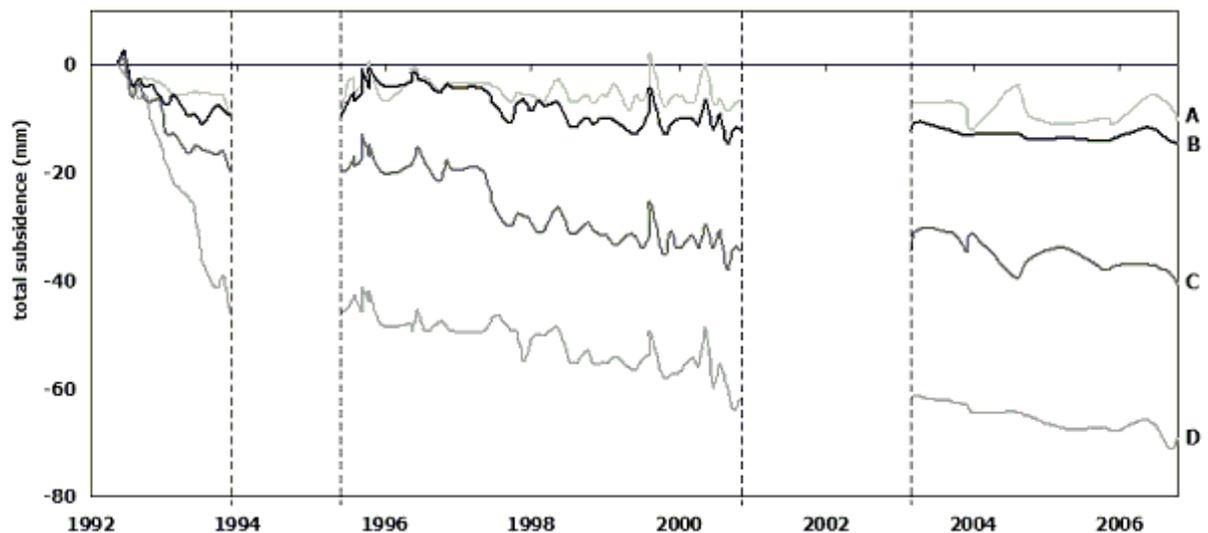
**Fig. 11** Cumulative subsidence at four selected points A – D in the Michal Mine area during the period 1992-2006.
