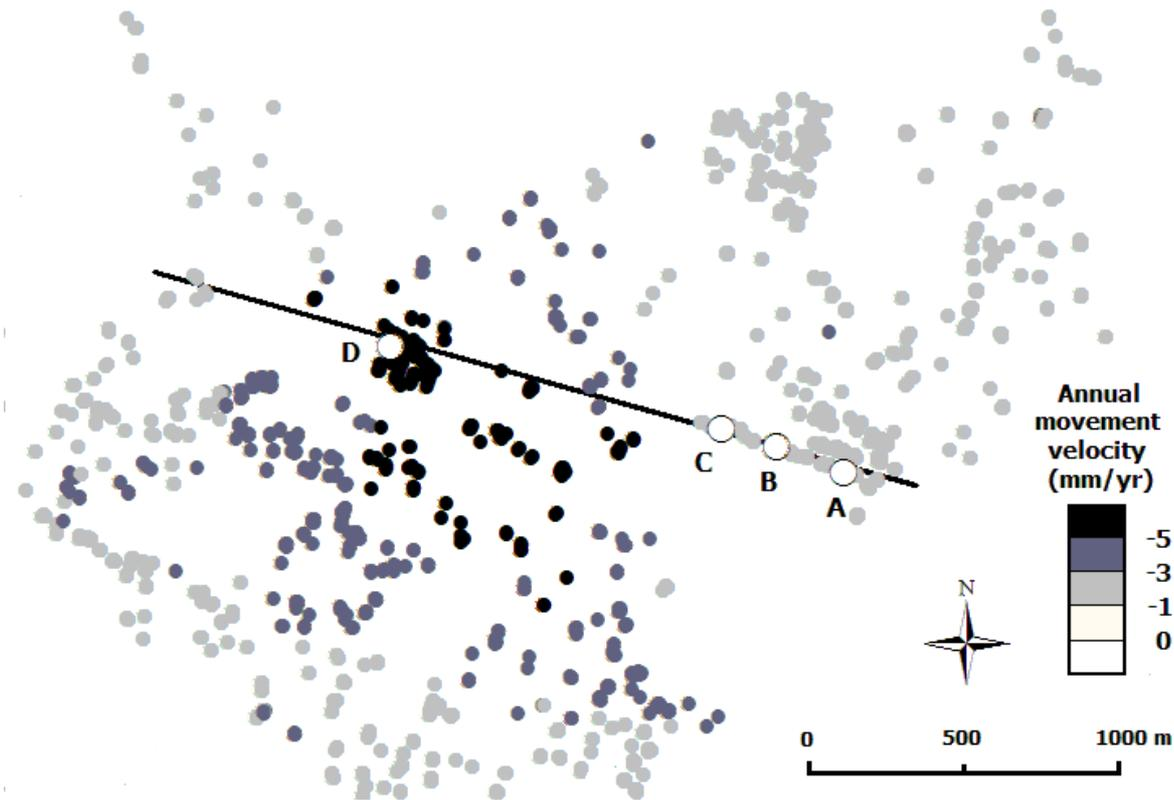
**Fig. 9** Distribution of PS in the Michal Mine area and their annual movement velocities during the 1995-2000 period (the cross-section is marked by a black line).
