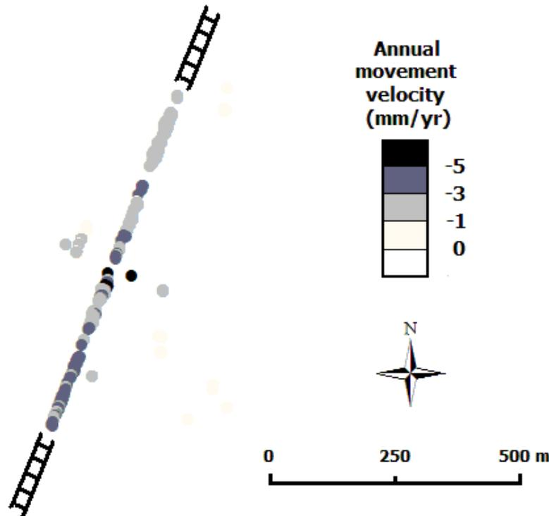
Fig. 6 Distribution of PS along the railway track in the locality Braník-Modřany and their annual movement velocities during the period 1995-2000 (direction of railway track is illustrated).
