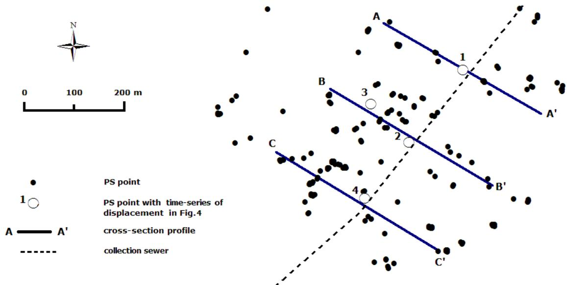
Fig. 3 Distribution of permanent scatterers (PS) along the collection sewer in the Stodůlky locality during the
