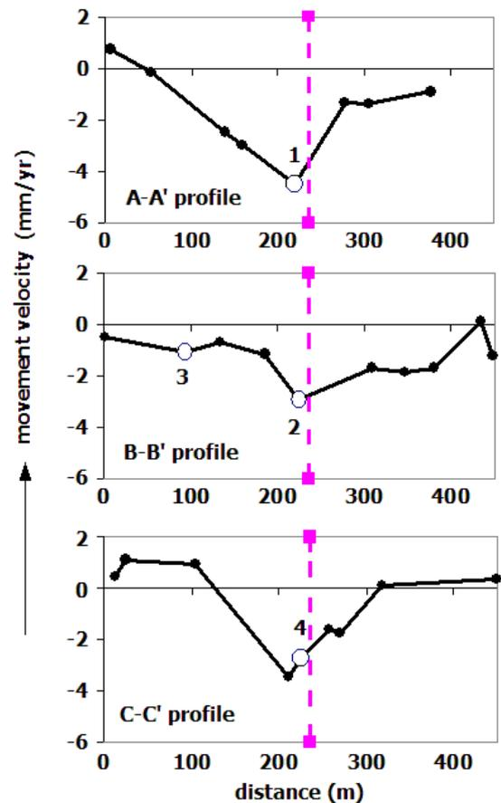
Fig. 5 Annual movement velocities for the nearest PS (marked in Fig. 3) along the cross-sections.
