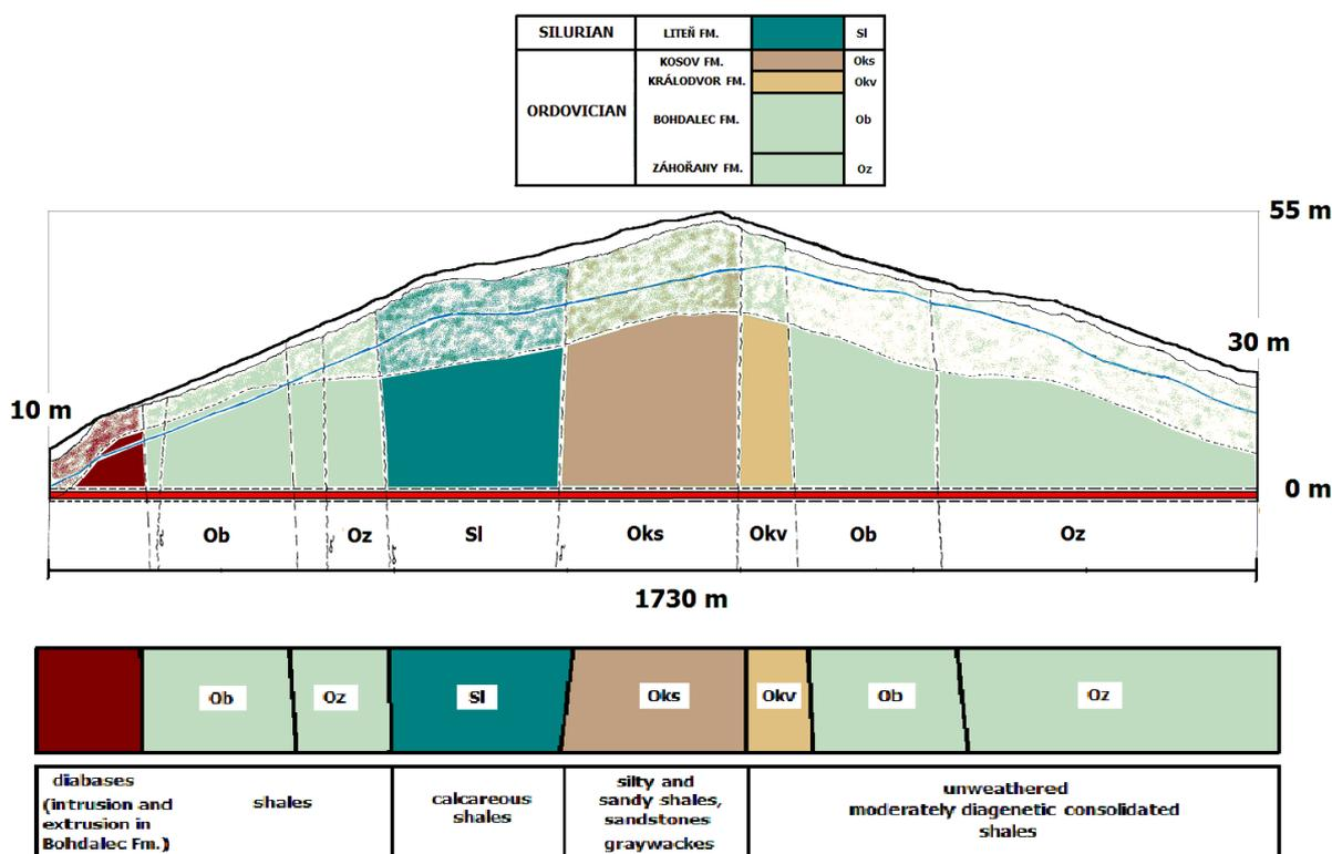
**Fig. 2** Geological section of the studied part of the collection sewer in the Stodůlky locality (adapted from Brandejs et al., 1996).
