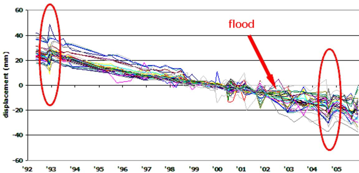
**Fig. 8** Time series of displacements for all PS for a selected section of the railway embankment in the Braník-Modřany locality (red ellipses mark "up and down" displacements for two periods: November 1992 – January 1993 and August – November 2004).
