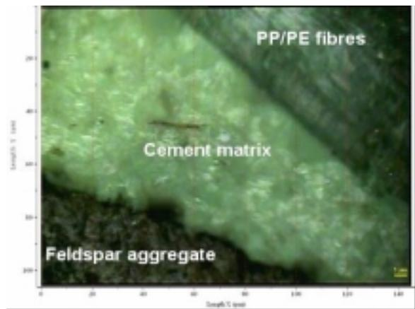
Fig. 2 Microphoto of concrete-PP/PE polymer analyzed area (magnification 10x)
