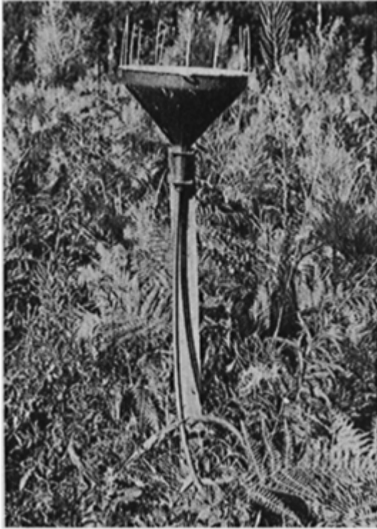
Figure 4.36 A bulk precipitation collector.
