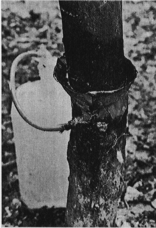
Figure 4.37 A stemflow collector.
