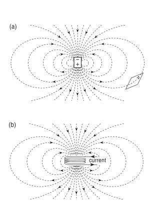
Figure 3.2: Magnetic field of a bar magnet and of a coil. (Musset and Khan 2000).
