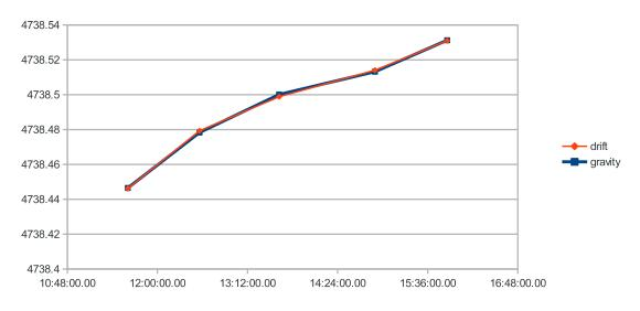
**Figure 2.14:** Drift correction. The blue line shows the gravity readings at the base station corrected for the free-air. The red line depicts the third-order polynomial fitted into the gravity readings. This polynomial will be used to estimate the drift values for the readings at individual stations.
