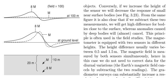
Figure 3.23: Anomalies at different heights of two dipoles (Musset and Khan 2000). Note the rapid decrease of amplitude of the shallower dipole.
