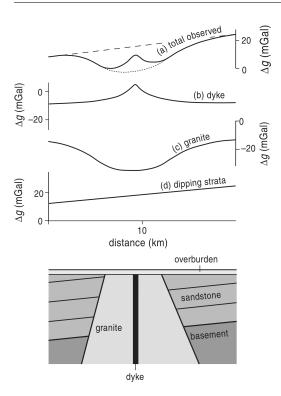
**Figure 2.15:** Illustration of regional and residual anomalies (Musset and Khan 2000). The observed gravity curve contains information about all geological structures (topmost curve). If we are looking for the dyke, then the anomalies due to the dipping strata and granitic pluton are not relevant to our research and we would like to remove them from the data to ease the interpretation.
