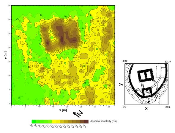
**Figure 4.21:** Resistivity survey over the former medieval fortress, Czech Republic. Wenner array with a 1 m inter-electrode distances was used, the resistivities were mapped in the  $1 \times 1$  m grid. The map of apparent resistivities (left) indicates the remnants of masonry as zones with increased resistivities. The interpreted ground-plan (right) shows the central tower, entrance with a gate, fortifications with adjacent smaller buildings and a ditch (dotted).
