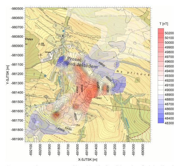
**Figure 3.25:** The magnetic image of basic dykes "Devil's walls", northern Czech Republic. A walking-mode caesium magnetometer (gradiometer) was used, the measured path is shown as a yellow line. The data from the top sensor are plotted here, the height of the sensor was 1.5 m. The magnetic highs are caused by the basic dykes, their NE boundary was formed by tectonic movements on the Lusatian Fault.
