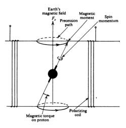
Figure 3.12: Proton precession (Telford et al. 1990).
