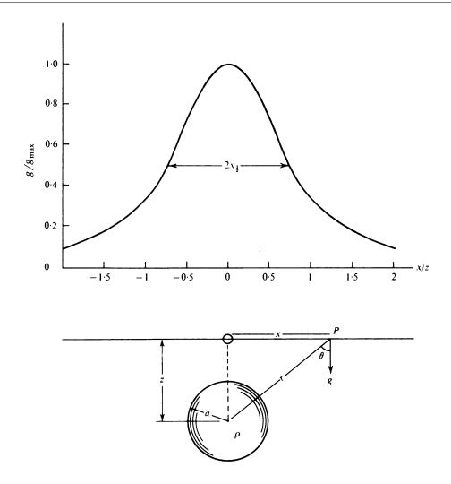
Figure 2.8: Gravity effect of a sphere (Telford et al. 1990)
