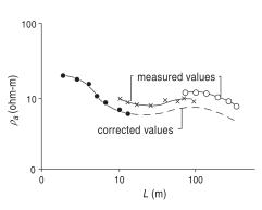
Figure 4.10: The individual branches of the resistivity curves could have offset if different potential electrode separations are used. Measuring several points with both offsets gives the redundancy necessary for correction. (Musset and Khan 2000.)
