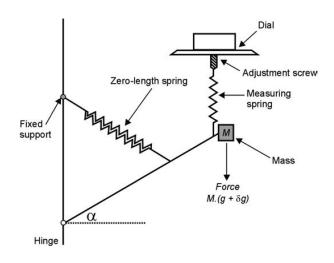
The gravity meters used for the geophysical prospection are the *astatic gravity meters* (Fig. 2.6), where the mass is hold by the measuring spring. Elongation of this spring is proportional to the gravity force pulling the mass. The older models of gravity meters used a dial to raise or lower the measuring spring to place the mass to a standard position. In modern gravimeters this is done automatically.
