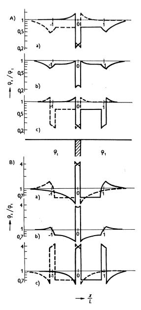
Figure 4.18: The resistivity curves over a thin dyke (Mareš and Tvrdý, 1984). a) Pole-dipole and reversed pole-dipole array. b) Schlumberger array. c) Dipole-dipole array. A) The case of a low resistivity dyke. B) The case of a high resistivity dyke. L is the length of the array.
