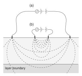
Figure 4.2: Change of a depth of penetration and of a volume sampled by the electric current for different separations of current elecetrodes (Musset and Khan 2000).
