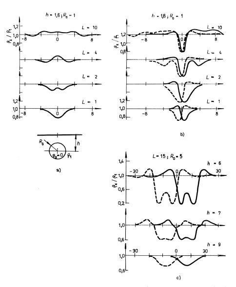
**Figure 4.17:** Resistivity curves over a conductive sphere (Mareš and Tvrdý, 1984). a) Potential array. b) Pole-dipole and reversed pole-dipole. Station is a midpoint of potential electrodes. c) Dipole-dipole array. Station is a midpoint of potential electrodes.  $R_0$  is a diameter of the sphere and h is the depth of its center.
