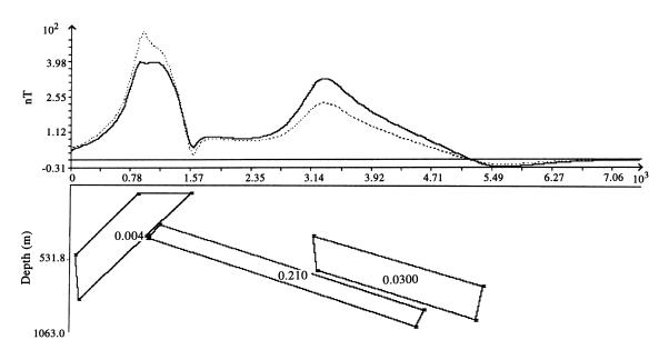
**Figure 3.19:** An example of magnetic profile build from the polygonal bodies. Calculated magnetic field anomaly is drawn with solid line and observed data are drawn using dotted line. Susceptibilities (in c.g.s. units) are displayed on bodies. (Cooper 1997).
