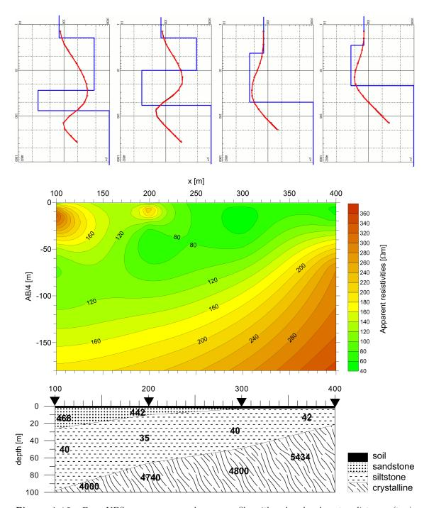
**Figure 4.16:** Four VES curves measured on a profile with a hundered meter distance (top). A resistivity pseudosection (middle) and an interpreted geological section (bottom) created from four VES curves on profile. The distance between individual VES points was 100 m. Interpreted resistivity values are added to the geological section.
