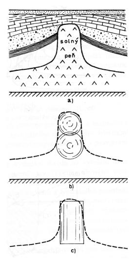
Figure 2.13: Approximation of a salt diapir (Mareš and Tvrdý 1984). a) A geological section of a diapir. b) An approximation of the diapir by two spheres. c) An approximation of the diapir by a vertical cylinder.
