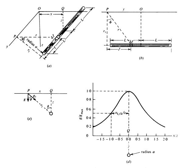
**Figure 2.9:** Gravity effect of a horizontal rod. a) Three dimensional view. b) Projection of the plane containing the rod and the y axis. c) Projection on the xz plane. d) Gravity profile along the x axis. (Telford et al. 1990)
