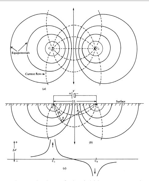
**Figure 4.1:** Equipotentials and current flow lines (paths) for two point sources of current on surface of homogeneous ground. (a) Plan view. (b) Vertical section. (c) Potential variation at the surface along a straight line through the point sources. (Telford et al. 1990.)
