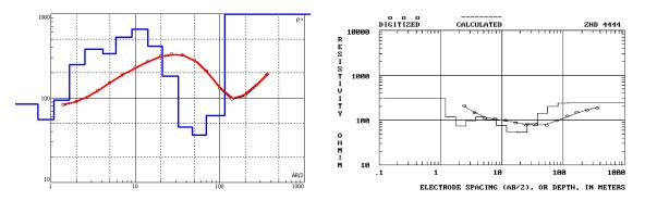
**Figure 4.15:** The VES curve from Fig. 4.14 interpreted using a gradient model (left) and a field example of the gradient environment (right) – a VES curve over a weathered granite. Each measured resistivity point represents one layer.
