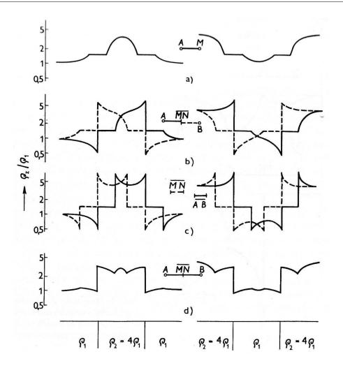
**Figure 4.8:** Apparent resistivity ( $\rho_a$ ) curves over a thick dyka (Mareš and Tvrdý 1984). a) Potential array. b) Pole-dipole and reversed pole-dipole array. c) Dipole-dipole array. d) Schlumberger array. The reference point (the point at which the measured resistivities are plotted) is in the middle of the potential dipole (or at the potential electrode in case of the potential array).
