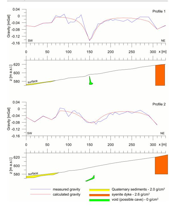
Figure 2.22: Gravimetry profiles showing possible occurrence of an underground cavity.
