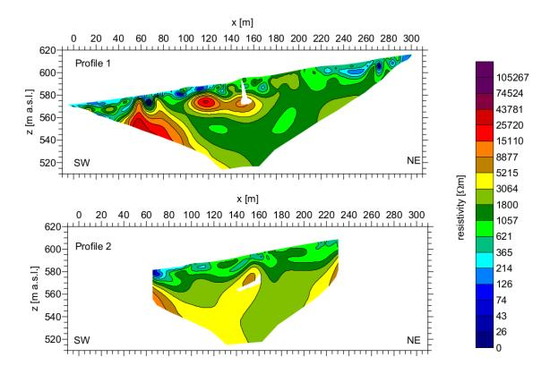
**Figure 2.23:** Resistivity cross-sections along the gravimetric profiles from the figure 2.22. Areas with high resistivities (yellow, brown and red colors) represents blocks of marble where the caves could evolve. White areas represent caves modeled according to the gravity data.
