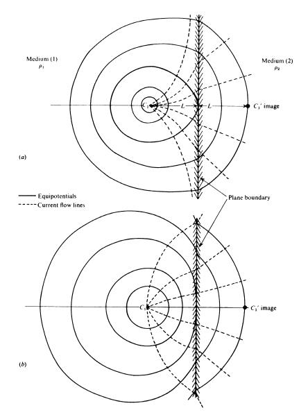
**Figure 4.5:** Distortion of equipotentials and current flow lines at a boundary between two media of different resistivities. (a)  $\rho_2/\rho_1 = 3$ . (b)  $\rho_2/\rho_1 = 1/3$ . (Telford et al 1990.)
