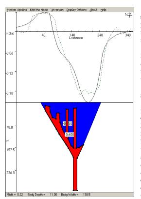
Figure 2.19: Modelling a maar-diatreme volcano as a set of 2.5D bodies. In the top graph the measured gravity curve (broken line) and computed curve for the current model (solid line) can be seen.
