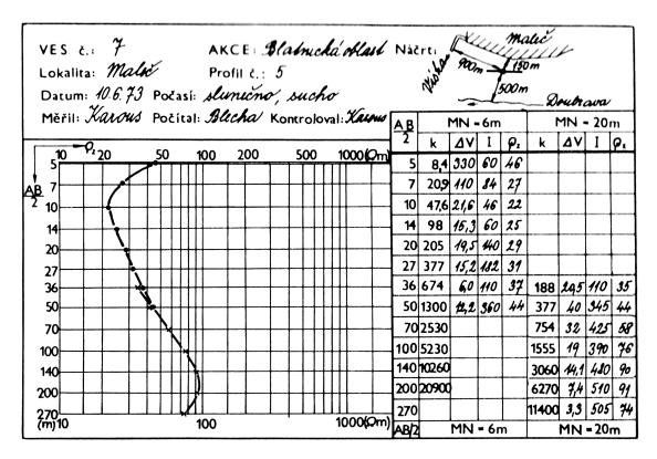
**Figure 4.9:** An example of the VES terrain chart (Mareš and Tvrdý 1984). For surveys mapping the near surface in more detail the first AB/2 (half of the current electrode separation) is usually 1 m and the starting MN (potential electrodes) distance is also 1 m. Note that the AB/2 distances are equidistantly sampled in a log scale. This is due to the exponential decrease of resolution with depth.
