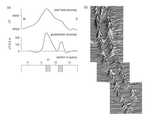
Figure 3.24: Gradiometer survey of the dolerite Butterton dyke, England (Musset and Khan 2000). The total field (a) does not reveal the fact that the dyke is in fact two thin parallel dykes. Nevertheless, this could be clearly recognised from the vertical gradient data. The set of parallel profiles maps a course of the dyke (b).
