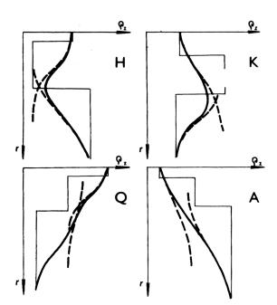
Figure 4.13: The four types of three layer curves and corresponding two layer cases (Mareš and Tvrdý 1984).
