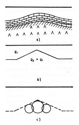
**Figure 2.12:** Approximation of an anticline (Mareš and Tvrdý 1984). a) A geological section of an anticline. b) A schematic representation with density distribution. c) An approximation of the anticline by three infinite horizontal cylinders.
