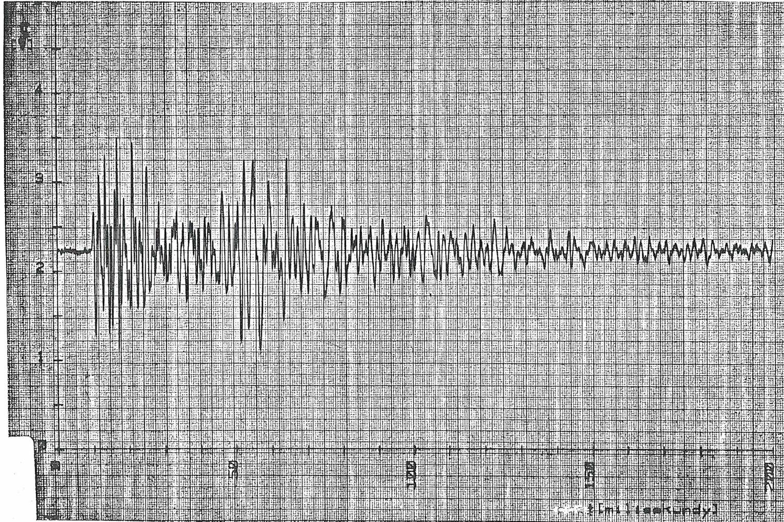
Fig. 1. A pair of seismoacoustic pulses recorded on magnetic tape.  $y$  - voltage on the GPIIIH geophone,  $x$  - time axis.
