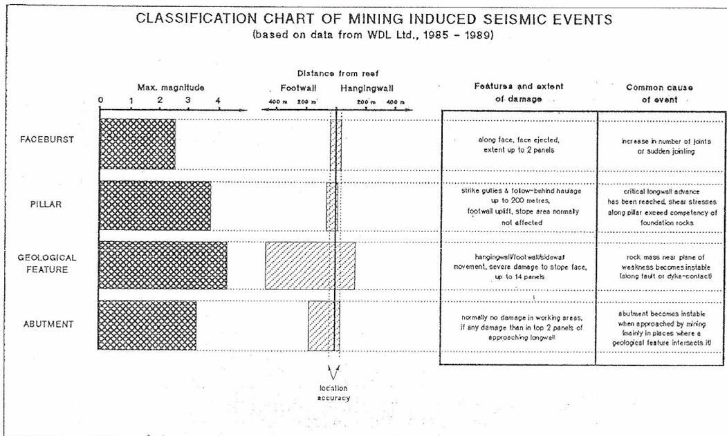
Fig.14 Categories of deep-mining-induced seismic events.
