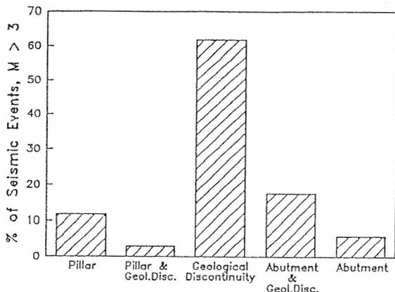
Fig.7 Large seismic events ( $M > 3$ ) and where they occur.
