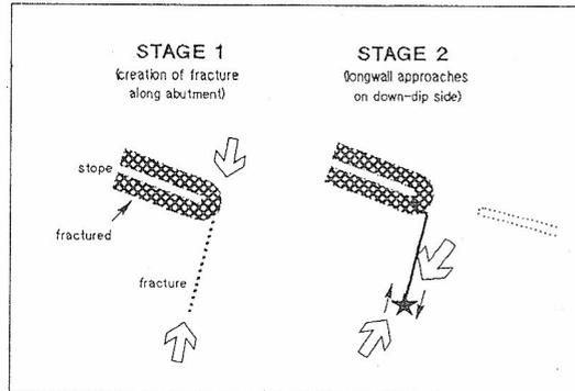
Fig.10 Proposed mechanism of an abutment failure.
