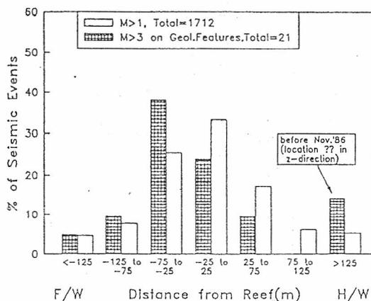
Fig.5 Seismic events and their distance from the reef.
