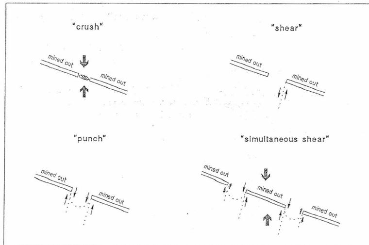
Fig.13 Proposed mechanisms of 'pillar'-failures.
