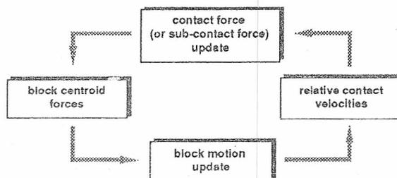
fig. 4 - 3DEC scheme calculations (after Hart, [1988])
