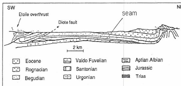
fig. 1- Geological cross-section of the basin
