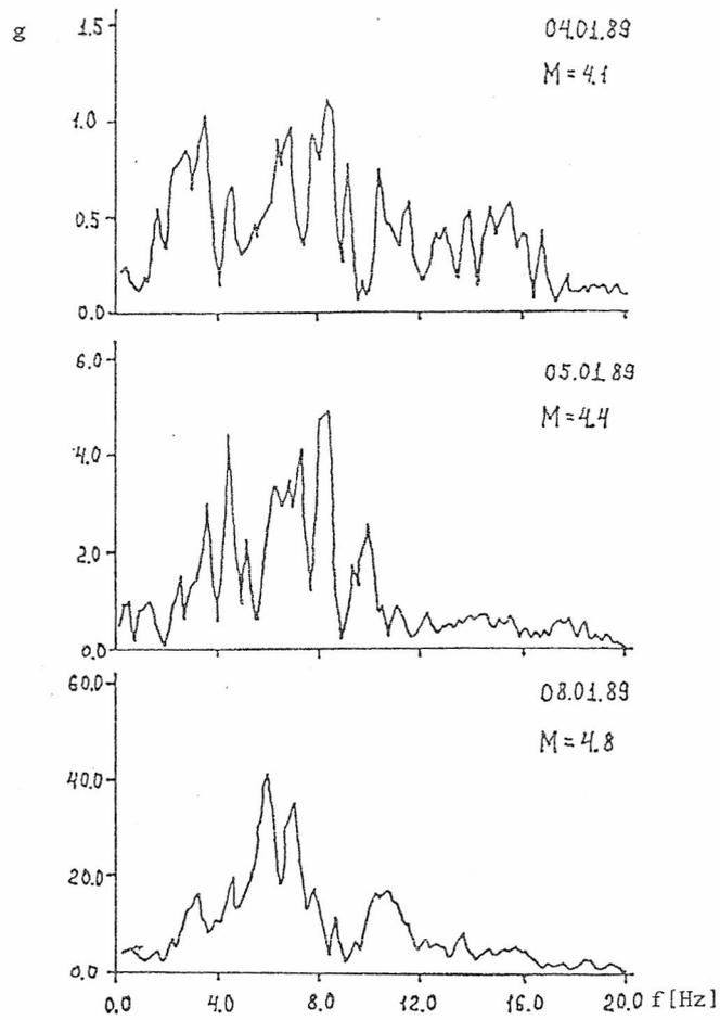
Fig. 11. Frequency spectra (lin/lin) of the accelerograms in Fig. 9. f - frequency, g - acceleration.
