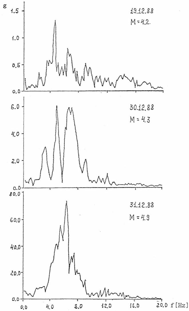
Fig.10. Frequency spectra (lin/lin) of the accelerograms in Fig. 8.  $f$  - frequency,  $g$  - acceleration.
