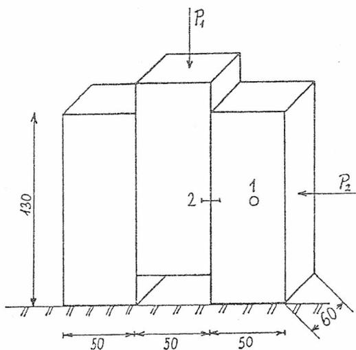
Fig. 1. Model set-up. Three magnesite blocks compressed by the confining force  $P_2$ ; central block is pressed against the two outer blocks by load  $P_1$ .
