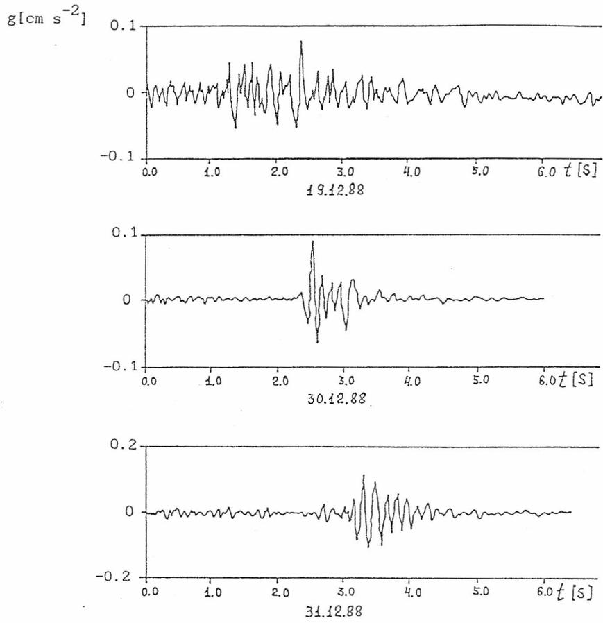
Fig.8. Three 1988 Spitak earthquake aftershocks, recorded by accelerometers, see the dates under seismograms,  $t$  - time,  $g$  - acceleration.
