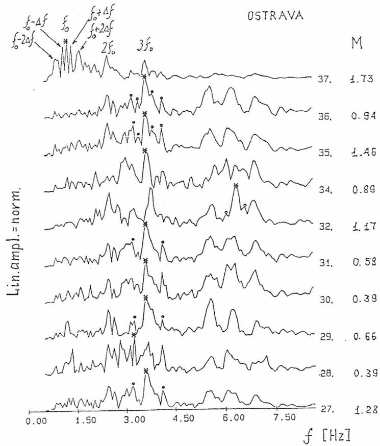
Fig. 7. Amplitude frequency spectra of the pulses from Fig. 6 in a lin/lin representation. By the asterisk the maximum values  $f_0$  in individual spectra are denoted, the point show the satellite local maxima  $f_0 \pm \Delta f_0$  or  $f_0 \pm 2\Delta f_0$ .
