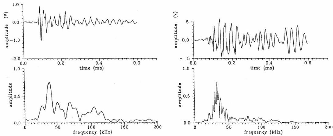
Fig. 4. Two seismoacoustic pulses from loaded magnesite model of a seismic source (upper part) and their amplitude spectra (lower part, rel. units).
