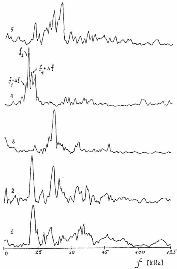
Fig. 3. Amplitude/frequency spectrum of the signals given in Fig. 2. The spectra patterns are given in linear normalized scale.  $f_1$  - maximum of the spectra in coherent stage of radiation.
