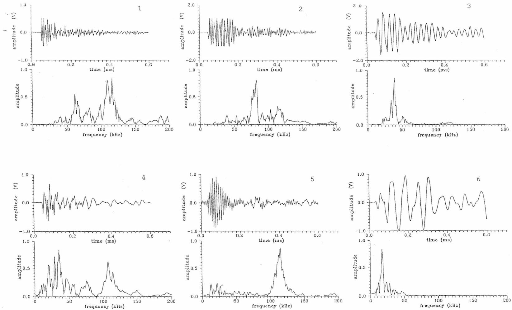
Fig. 5. Three acoustical pulses, 1, 2 and 3 from loaded fine grained sandstone source model and their amplitude spectra, see the row under the pulses 1-3. In the lower half of the figure three acoustical pulses 4, 5 and 6 from loaded coarse grained sandstone source model are shown together with their amplitude spectra (bottom row). Both the samples were taken from the Kladno coal region.
