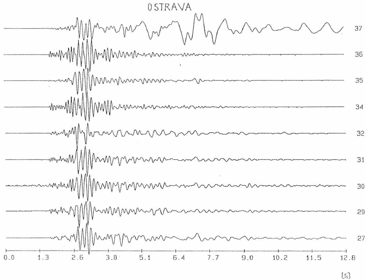
Fig. 6. Seismic records of nine rockburst events taken from the Ostrava coal region, which were selected from one locality in a time interval Apr-Nov 1988. Time is given in seconds, the amplitudes are normalized.
