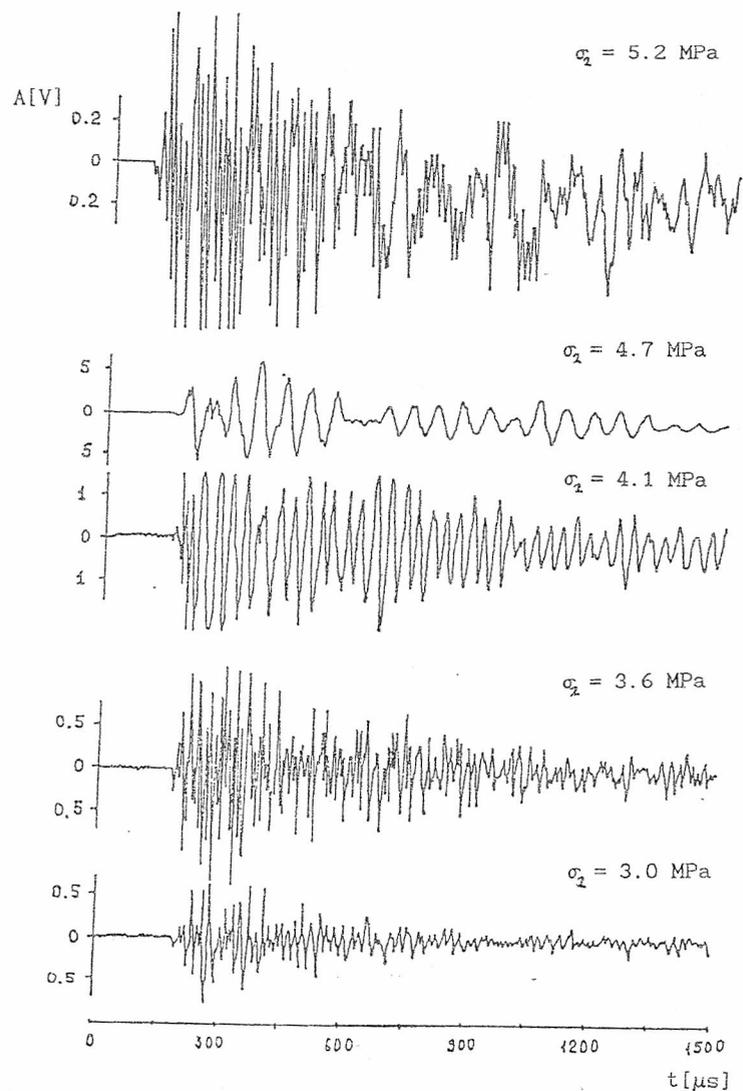
Fig. 2. Form of the stick-slip signals radiated in 5 different levels of confining pressure  $\sigma_2$ .
