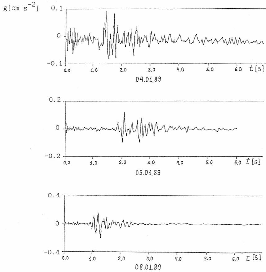
Fig.9. Three 1989 Spitak earthquake aftershocks recorded by accelerometers, see the date under seismograms.  $t$  - time,  $g$  - acceleration.
