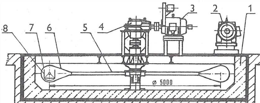
FIG 1. Scheme of centrifuge
