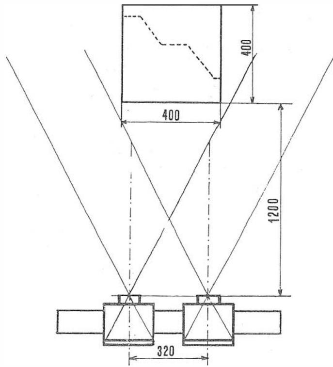
FIG 2. Scheme of photogrammetric measurements
