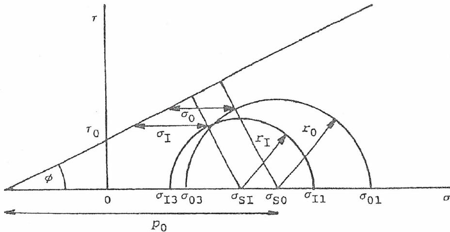
FIG. 1. Scheme of the Mohr diagram for the initial stage and case I of stress distribution.
