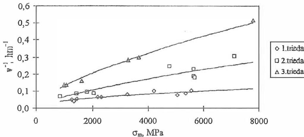
FIG. 1. The relationship between the inverse value of the actual penetration rate of drilling and the indentation hardness at drilling by impregnated tools
