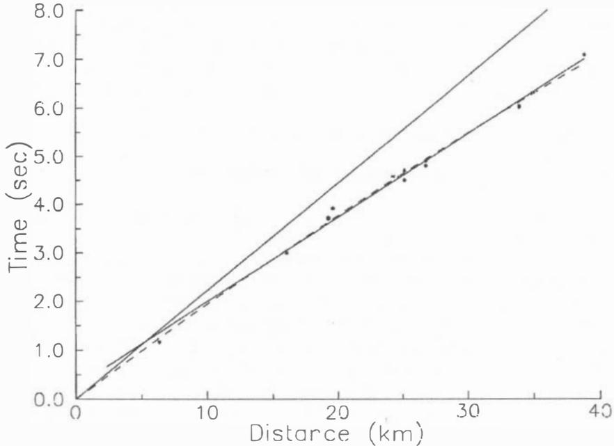
FIG. 3. Observed travel times (points) and their approximation by the direct and head wave travel times for model D (solid lines) and by the second order polynomial (dashed line)
