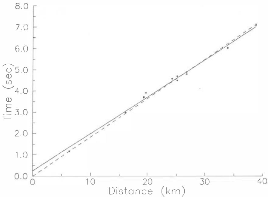
FIG. 2. Observed travel times (points) and their straight-line approximations: the solid line shows the line given by formula (1), the dashed line shows the line given by formula (2)
