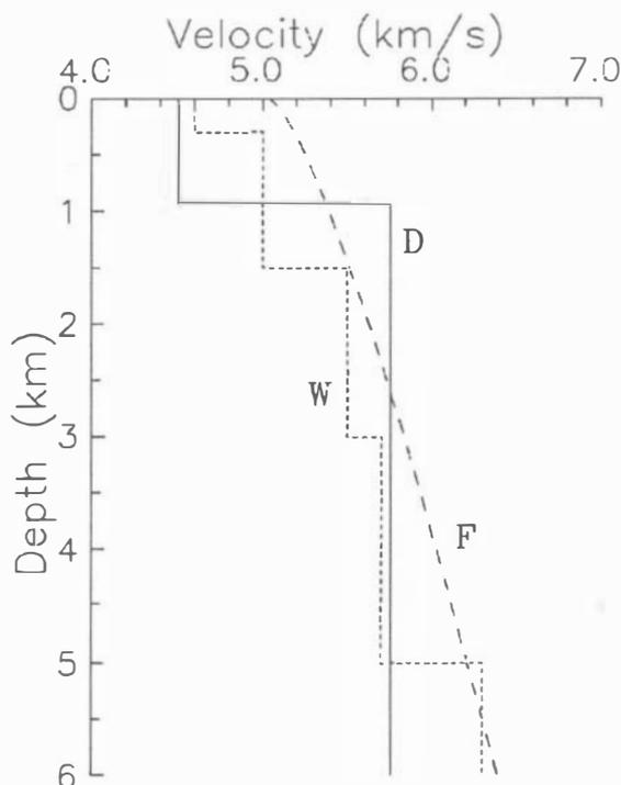
FIG. 4. *P*-wave velocity–depth distribution for model D (solid line), model F (dashed line), and model WB95 (dotted line)
