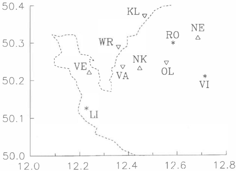
FIG. 1. The position of the shot-points (\*), digital seismic stations ( $\Delta$ ) and analog seismic stations ( $\nabla$ ). For the abbreviations see Tab. 1
