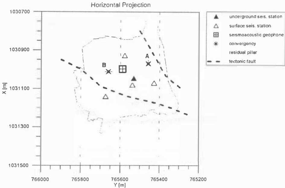
FIG. 1. Schematic map of Kladno II mine situation. Horizontal projection of monitoring method location
