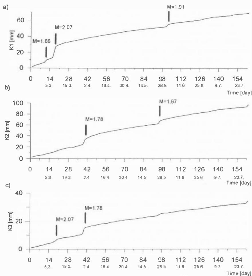
FIG. 5. Convergency time series - measuring point B-K1 (a), point A - K2, K3 (b,c)
