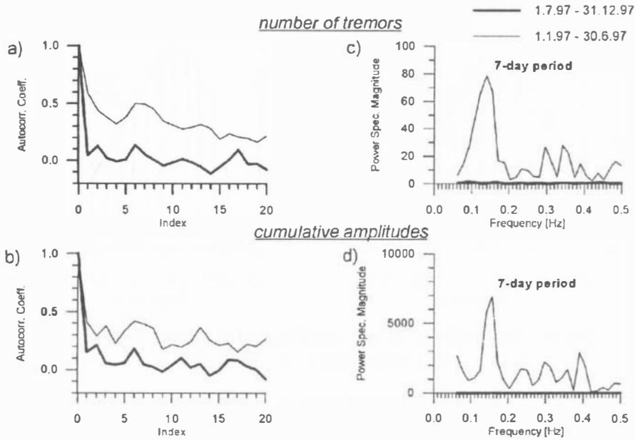
FIG. 9. Correlation function of number of tremors (a) and cumulative amplitude (b) and power spectrum density of number of tremors (c) and cumulative amplitude (d). Thin line depicted time interval during mining activities and thick line after stopping mining
