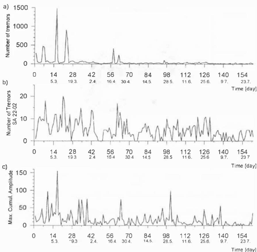
FIG. 6. Seismoacoustic time series (a), seismoacoustic time series selected from 22 to 02 hour (b), seismic time series of cumulative amplitude (c)
