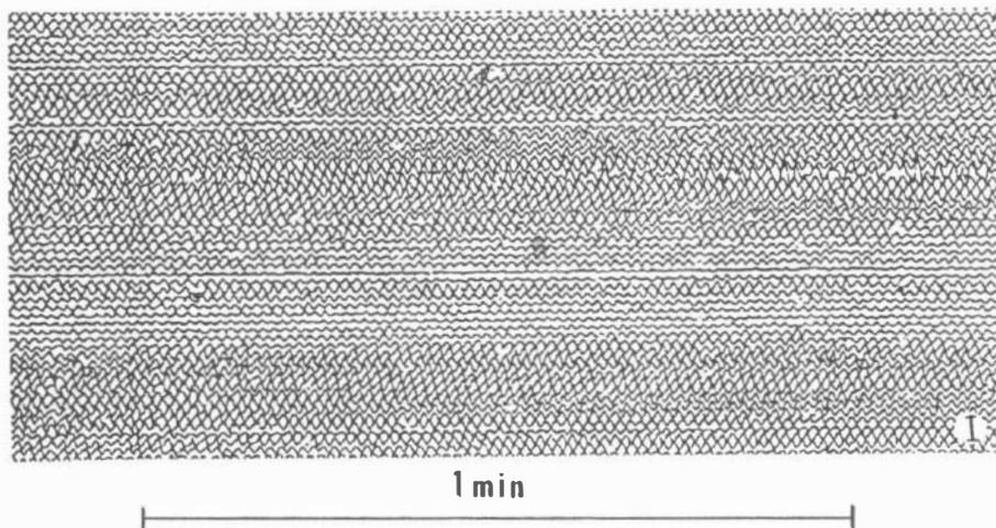
FIG. 11. Wave pattern recorded by the vertical short-period seismograph at the seismic station Ostrava-Krásné Pole (OKC). The bar in the right lower corner represents the displacement amplitude of  $A = 100$  nm.
