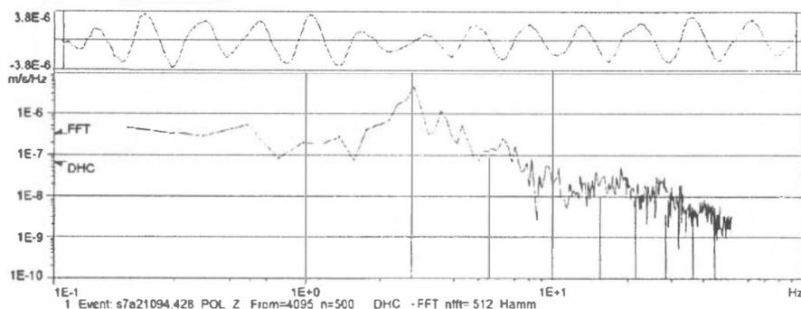
FIG. 3. Seismogram section (vertical component) of vibrations caused by a freight train passage recorded at the distance of about 800 m near village Polanka (top) and the corresponding frequency spectra (FFT and DHC algorithm) (bottom).
