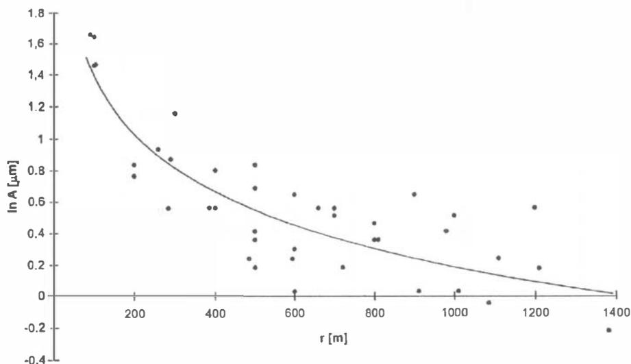
FIG. 8. Experimental amplitude–distance curve of the vertical component of vibrations with periods of  $T \approx 0.5$  s generated by large piston compressors.
