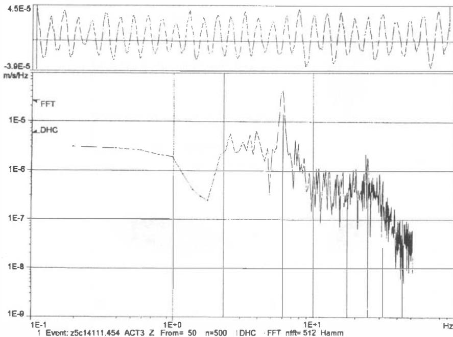
FIG. 9. Spectral analysis of the vertical component of vibrations induced by the compressor operation.
