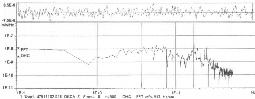
FIG. 2. Seismogram section (vertical component) of vibrations induced by local traffic and recorded at the station Ostrava-Krásné Pole (OKC) (top) and the corresponding frequency spectra (FFT and DHC algorithm) (bottom).
