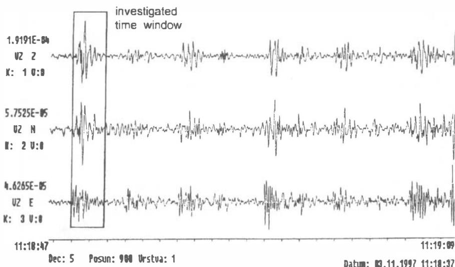
FIG. 5. Three component seismograms of vibrations induced by a forging shop operation made at an epicentral distance of  $r \approx 175$  m.
