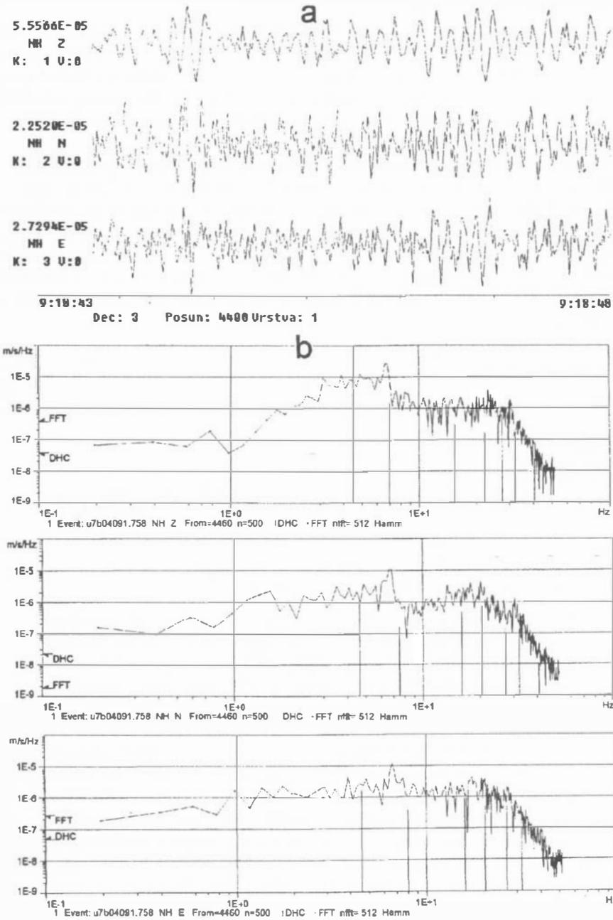
FIG. 4. Three component seismograms of vibrations generated by a freight train passage (a) in the Nová huť area and corresponding FFT spectra (b).
