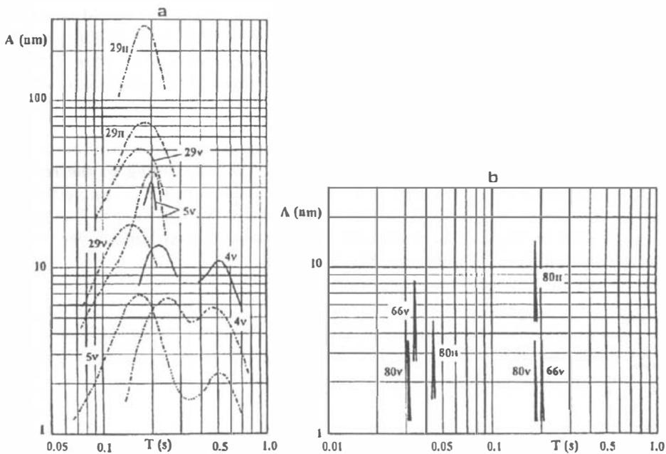
FIG. 1. Level of seismic noise generated by man-made sources. **a** – moving source (train), **b** – stationary source (water-work pump). — daytime observation, - - - night observations, 4, 5, 29, 66 and 80 denotes no. of the site along the respective profile, V or H (vertical or horizontal component) (after Holub 1977).
