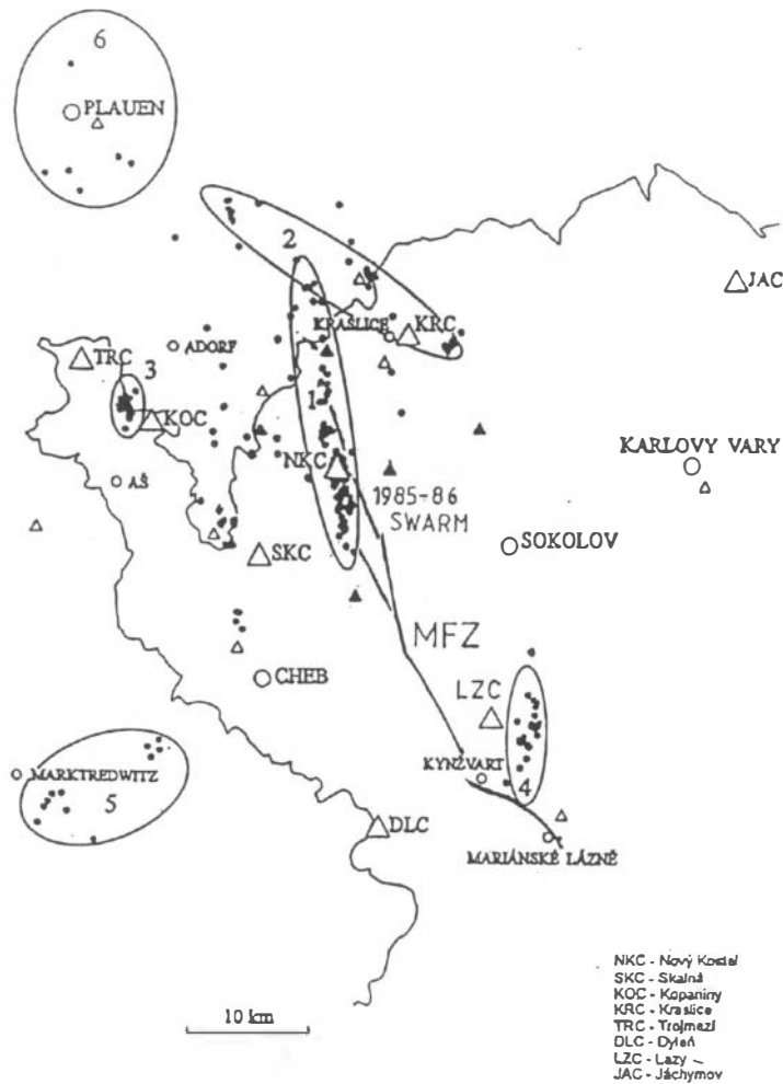
FIG. 3. WEBNET (Western Bohemian Network) – positions of seismic stations: \Delta – stations of the Geophysical Institute AS CZR and Institute of Rock Structure and Mechanics AS CZR; \blacktriangle stations of the Institute of Earth Physics, Masaryk University Brno; \bullet earthquake foci (1–6 areas, Horálek et al., 1996); MFZ – Mariánské Lázně fault zone
