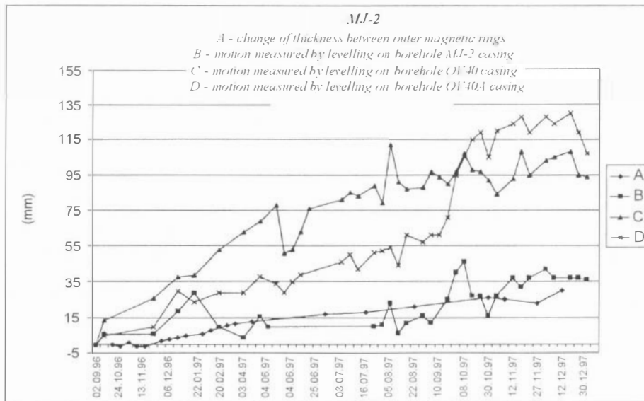
FIG. 15. Borehole MJ2 — distance alteration between marginal magnetic rings in comparison with motion of MJ2, OV40 and OV40A borehole casing heads
