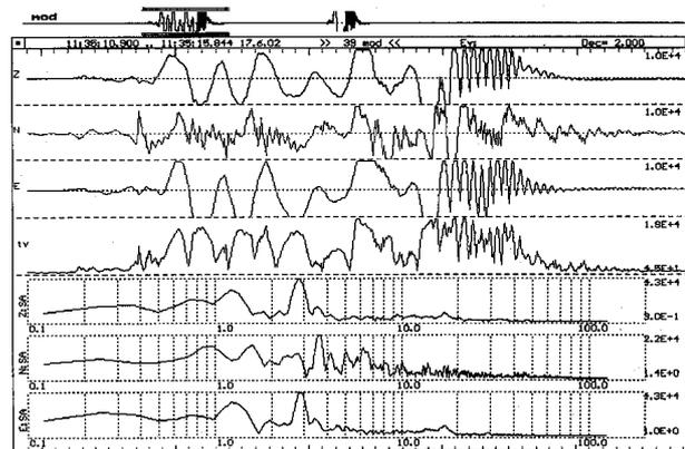
**Fig. 12** Record of simulated shock. The vibration speed components ( $\mu\text{m/s}$ ) are up and the frequency spectrum (Hz) is below.
