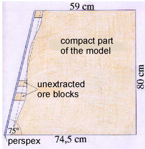
**Fig. 1** Model design: side-view.
