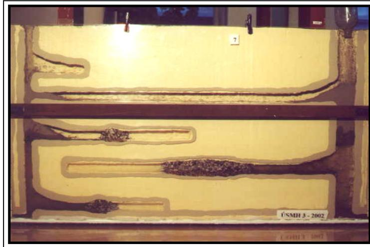
**Fig. 15** Condition of the model after light ash had been poured into both shafts
