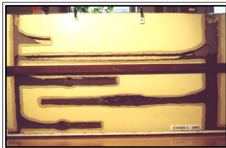
**Fig. 14** Penetration of the light ash beyond the modelled caving falls
