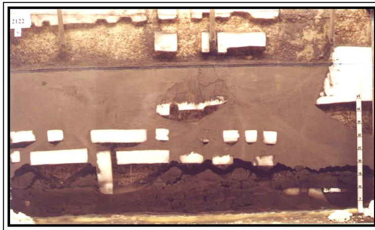
**Fig. 5** Gradual soaking of the light ash in the model
