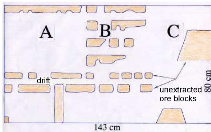
**Fig. 2** Model design - blocks A, B, C and distribution of ores in place in the model space.
