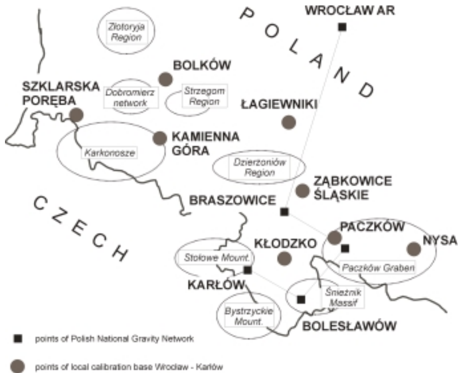
Fig. 1 Schematic representation of the PNGN points and points of the local reference network set up in 1992 against the background of the studied areas
