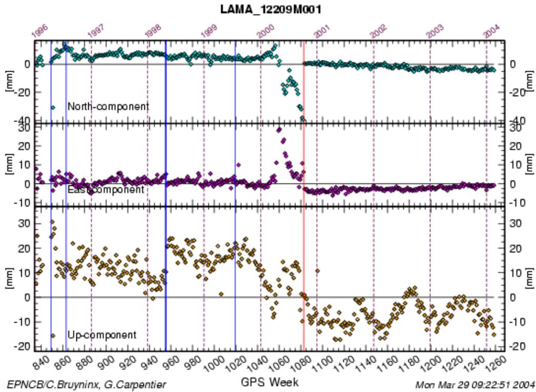
**Fig. 3** Time series of site coordinates transformed to north, east and up components at the permanent site LAMA (Bruyinx and Carpentier, 2004)
