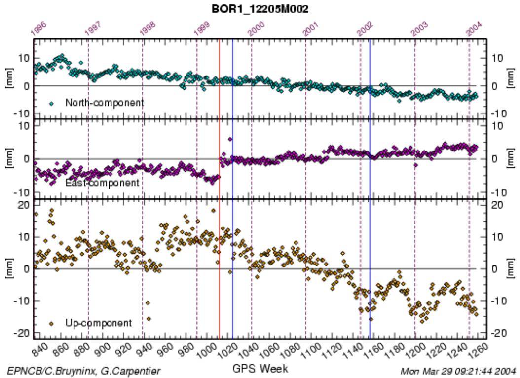
Fig. 1 Time series of site coordinates transformed to north, east and up components at the permanent site BOR1 (Bruyinx and Carpentier, 2004)
