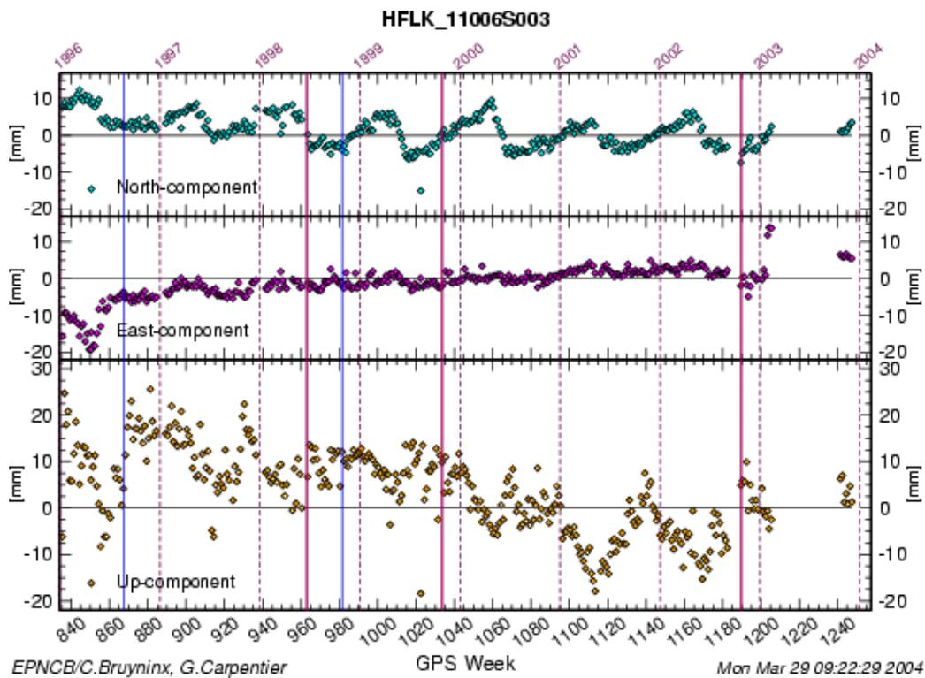
**Fig. 4** Time series of site coordinates transformed to north, east and up components at the permanent site HFLK (Bruyinx and Carpentier, 2004)
