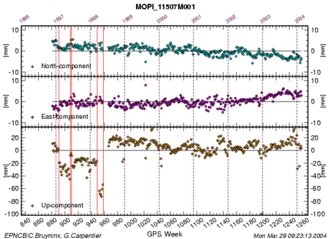
Fig. 2 Time series of site coordinates transformed to north, east and up components at the permanent site MOPI (Bruyinx and Carpentier, 2004)
