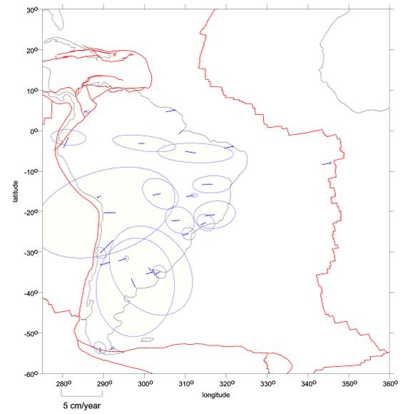
**Fig. 10** Residual motions with 2.5 sigma error ellipses, SOAM plate
