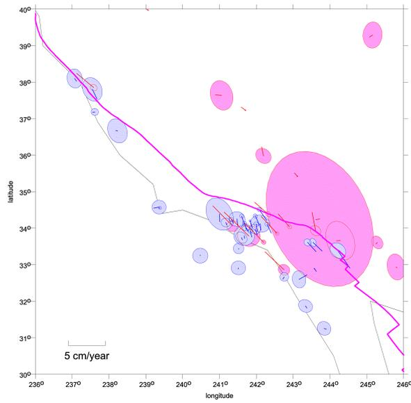
**Fig. 9** Residual motions with 2.5 sigma error ellipses, NOAM (red) and PCFC (blue) plates, California part only
