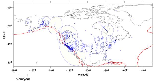
**Fig. 8** Residual motions with 2.5 sigma error ellipses, NOAM plate
