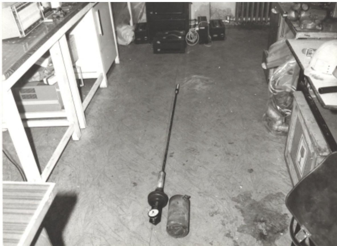
Fig. 12 Photograph of a deep probe
