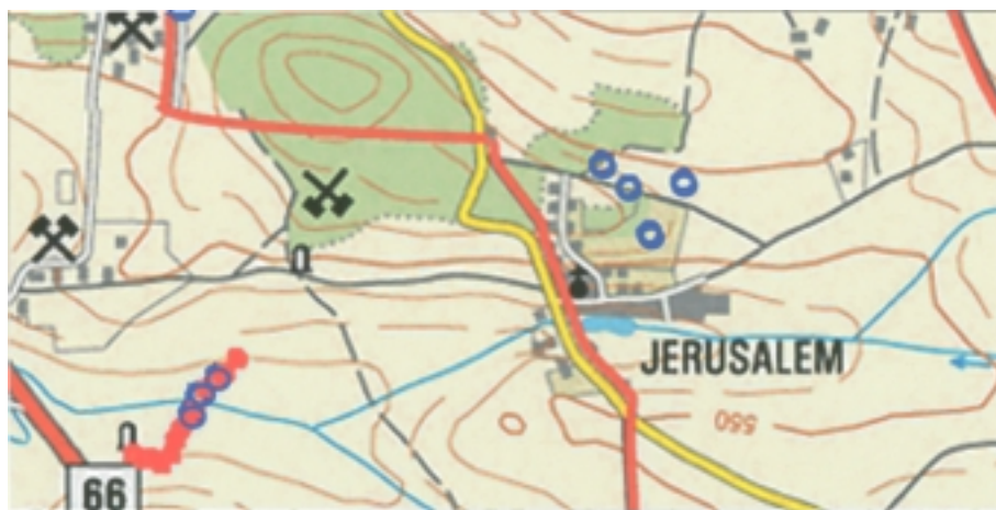
Fig. 10 Levelling traverses in the Brod and Jeruzalém areas
