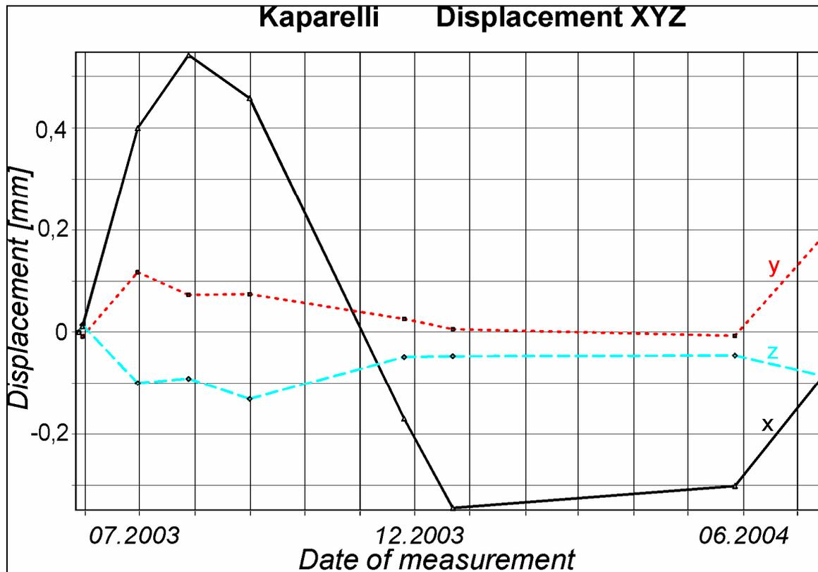
**Fig. 5** Displacement – Time diagram for site Kap2 along the Kaparelli Fault. X direction measures displacement across the fault plane, Y direction along the fault plane and Z along the vertical direction, respectively.
