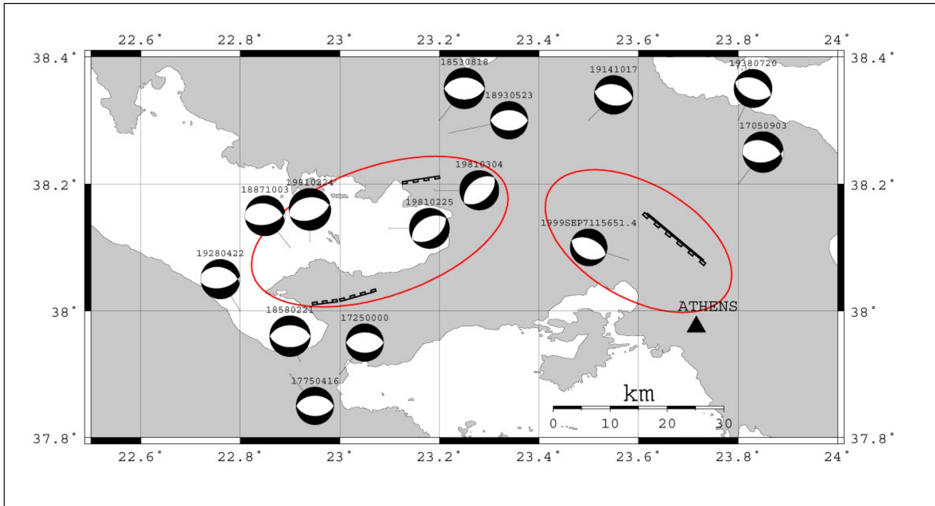
**Fig. 1** Seismicity map of the eastern Gulf of Corinth and Attica regions since 1700 showing events  $\geq 5.9$ Ms. Ellipses indicate rupture zones of the 1981 and 1999 earthquakes. These zones differ in both location and trend (NE-SW for Corinth vs. NW-SE for Attica). Beachballs indicate fault plane solutions with black colour indicating compression.
