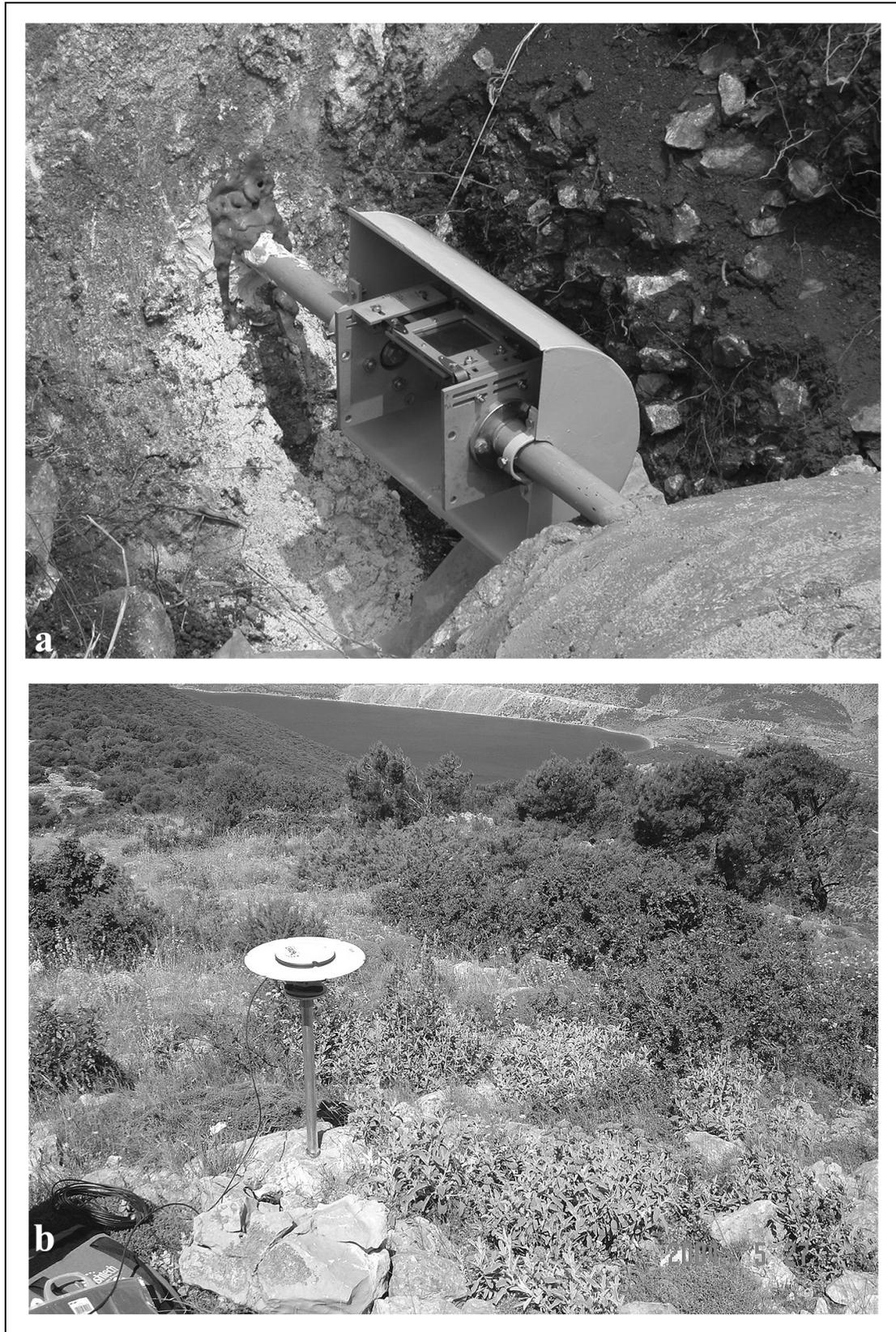
**Fig. 4** Field photographs of deformation monitoring instruments. a) TM-71 installation inside trench Kap2 (May 2003; see Fig. 2 for location). b) GPS antenna and receiver in operation near the Agios Vasilios Bay (Station TAPS; May 2004).
