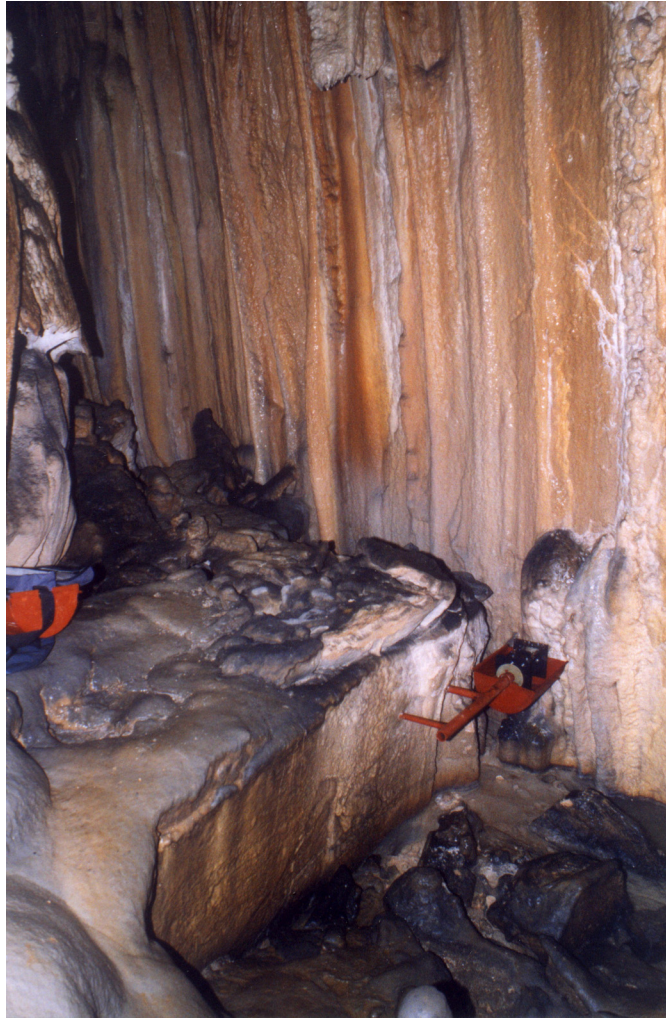
Fig. 1 TM71 device installed across the fault in Postojna cave system (Postojna 1)
