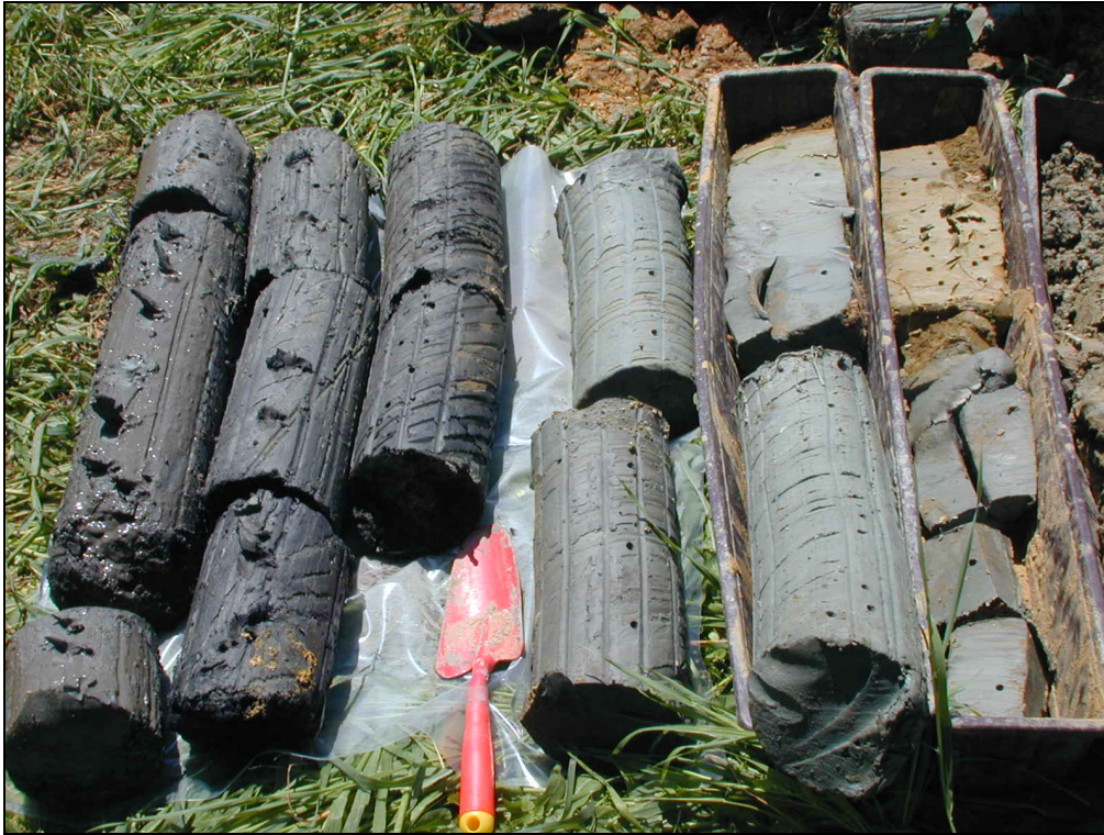
Fig. 1 Miocene clays with organic matter (J204A borehole, depth of 7.0-8.0 m)
