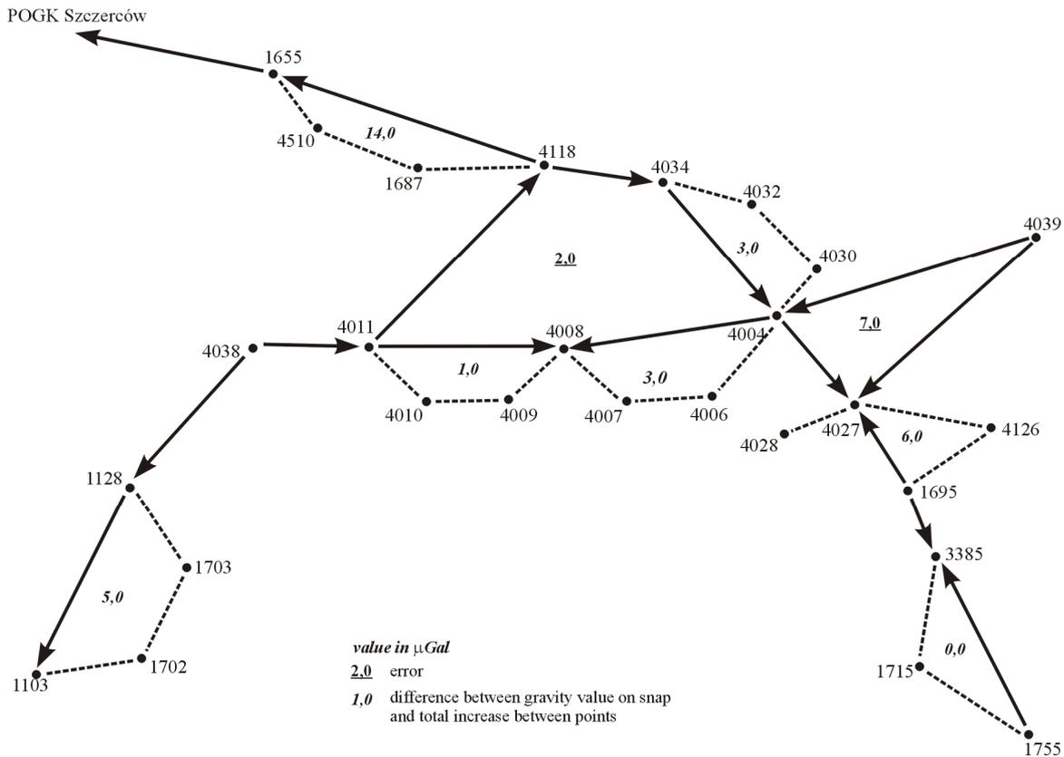
Fig. 7 Gravity measurement diagram on “Dębina” salt dome
