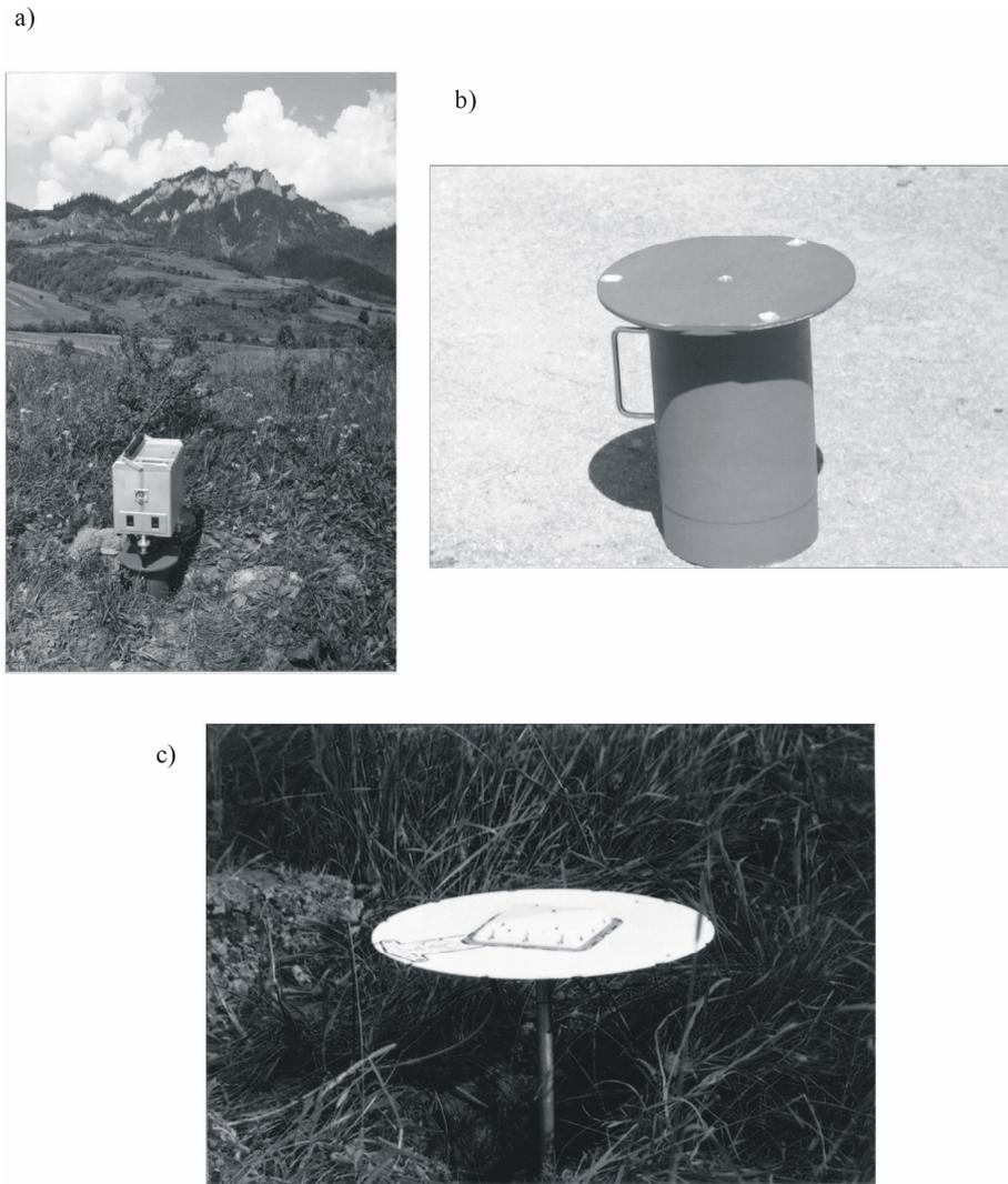
**Fig. 3** Gravity and GPS measurement and using devices a) gravity meter on stand, b) stand, c) GPS aerial
