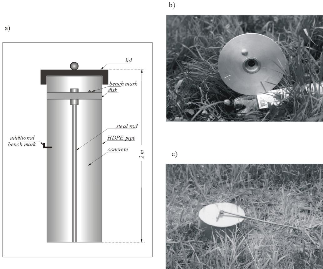
**Fig. 2** Construction of geodynamic station, a) station cross – section, b) disc appearance, c) lid
