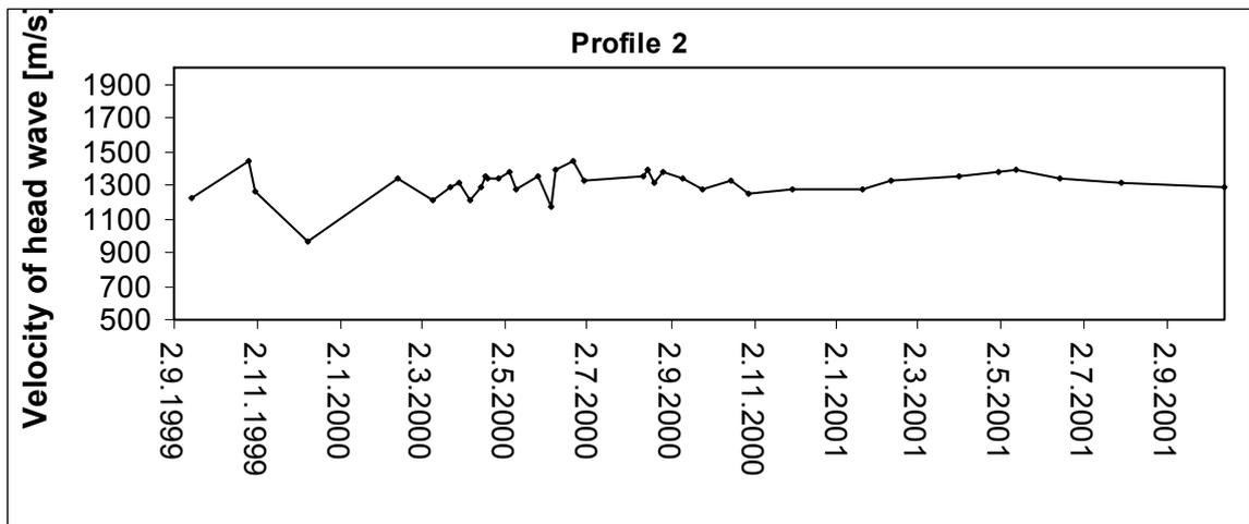
Fig. 3 Variation in velocity of head wave in profile No.2 perpendicular to the direction of exploitation.
