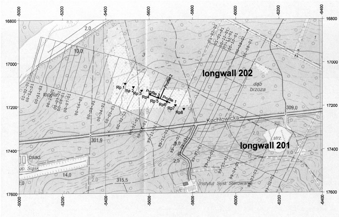
**Fig. 1** Scheme of research area with surface projection of exploited longwalls in consequent time period (coordinates in Sucha Góra Reference Frame in meters).
