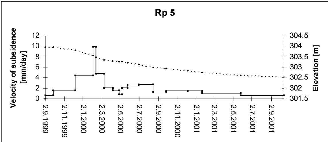
Fig. 8 Subsidence measured at benchmark Rp 5.
