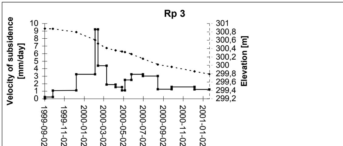
Fig. 11 Subsidence measured at benchmark Rp 3.
