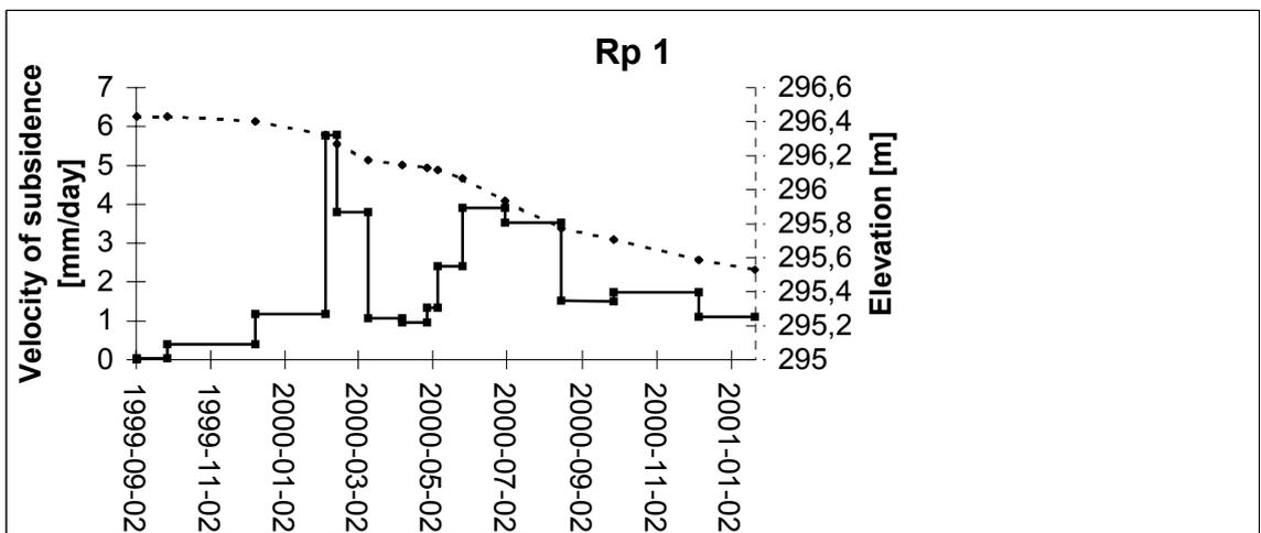
Fig. 10 Subsidence measured at benchmark Rp 1.
