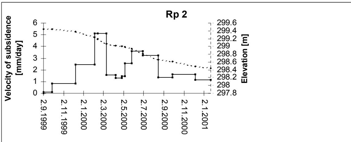
Fig. 9 Subsidence measured at benchmark Rp 2.
