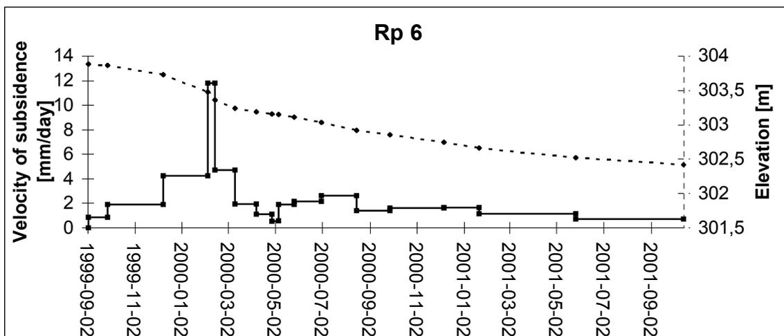
Fig. 7 Subsidence measured at benchmark Rp 6
