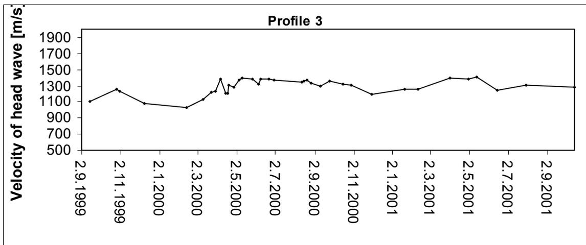
Fig. 4 Variation in velocity of head wave in profile No. 3 in accordance with the direction of exploitation.
