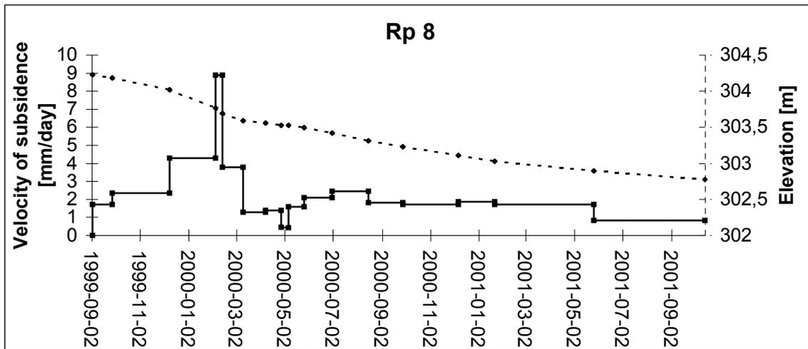
Fig. 5 Subsidence measured at benchmark Rp 8.
