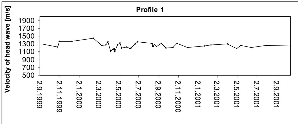
Fig. 2 Variation in velocity of head wave in profile No.1 in accordance with the direction of exploitation.
