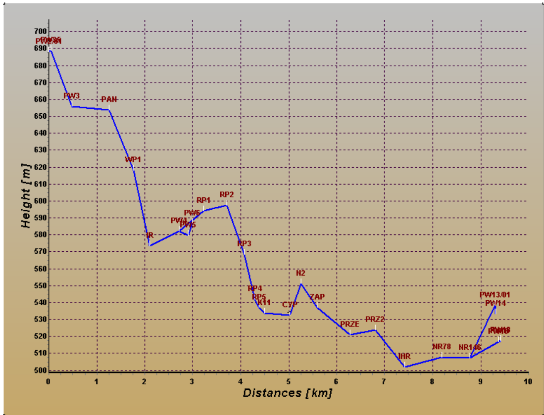
Fig. 2 Vertical profile of the control-line; significant differences in elevations can be seen; they caused terrestrial precise leveling very heavy
