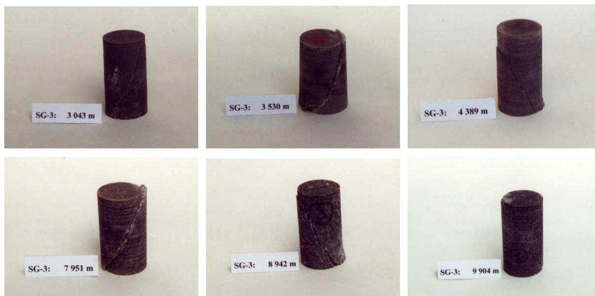
**Fig. 4** Disturbed core specimens after unconfined compressive test
