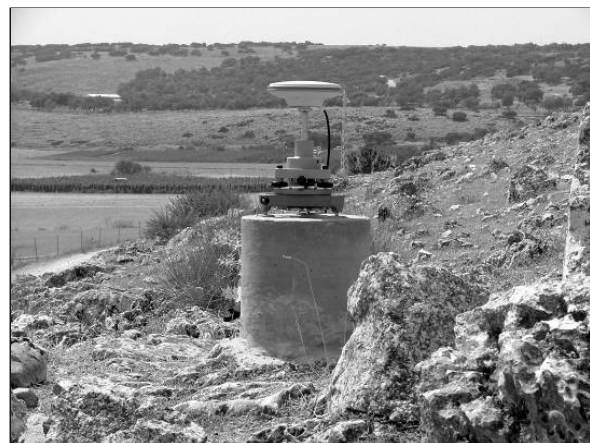
Fig. 6 Concrete pillar for GPS measurement at site 800 of the Zafarraya network.
