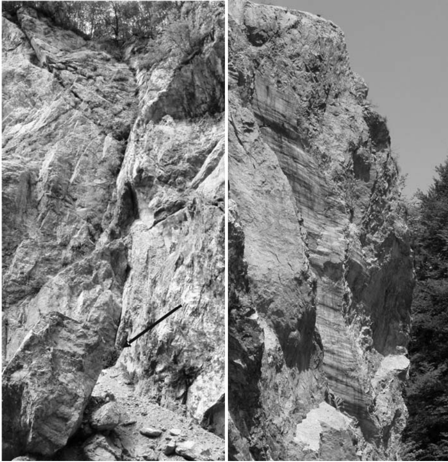
Fig. 5 Left: the crack in the inner zone of the Idrija fault in the Učja valley. The arrow shows the location of TM 71 instrument. Right: The exposure of the fault plane 50 m from the crack shown in the left figure with clear striations indicating subhorizontal movements.
