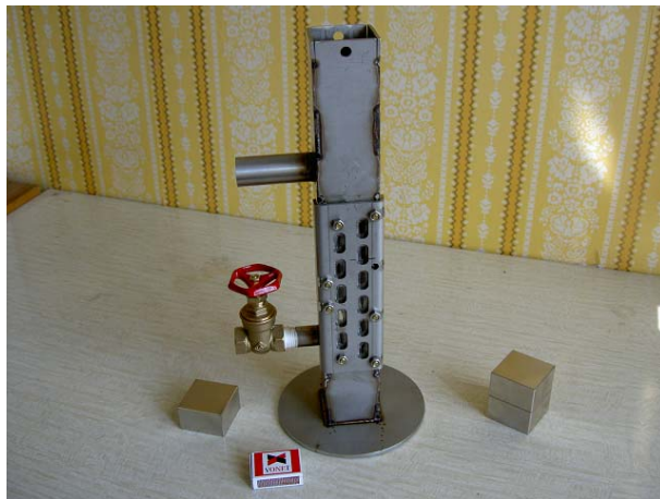
Fig. 4 Equipment for assembling small blocks of magnets with dimensions of 0.05 x 0.05 x 0.03 m.
