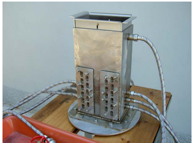
Fig. 5 Equipment for assembling large magnetic blocks from magnetic plates.
