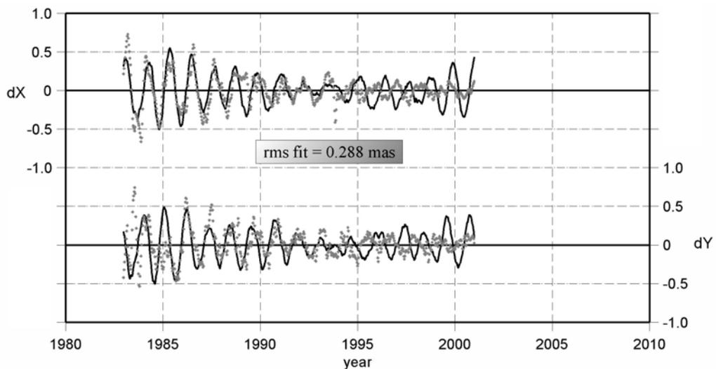
**Fig. 5** Observed and integrated celestial pole offsets with ERA40 AAM + OMCT OAM.
