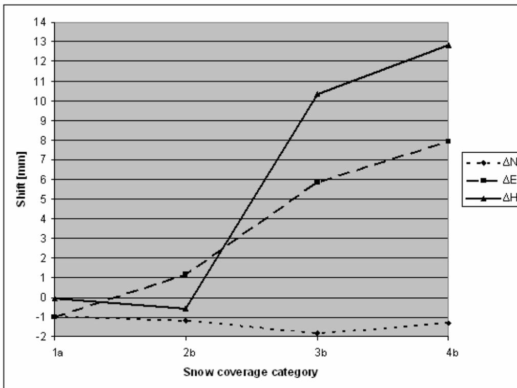
Fig. 9 Shifts in position of the observatory SNEC for three components.
