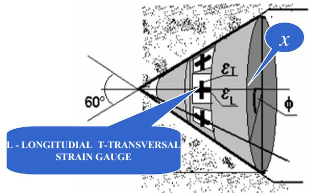
**Fig. 1** Scheme of siting of the gauge sensors on conical body of probe.
