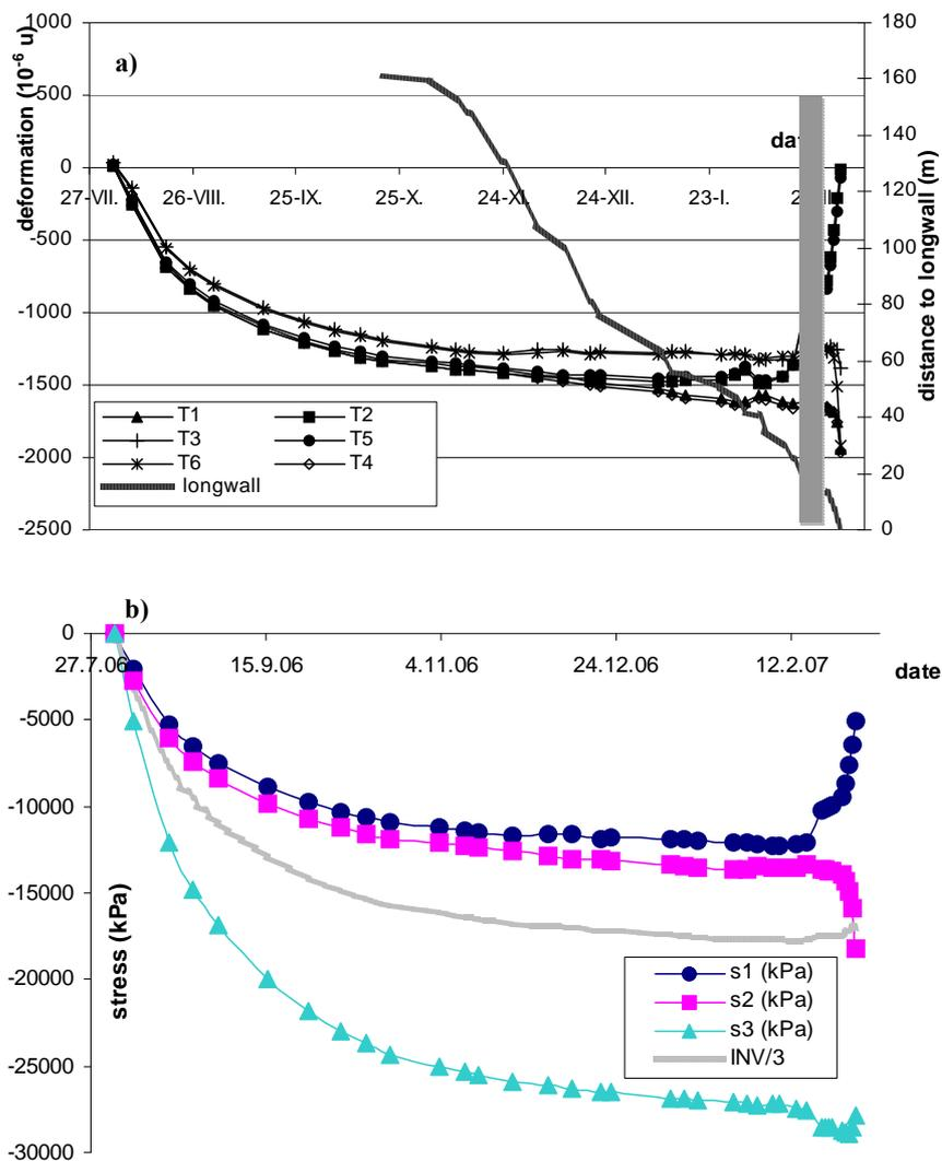
Fig. 5 Probe 1<sub>9</sub>. a) record of deformation measurement on the gauges „T“-type, b) calculated stress representation of the gauges deformations.
