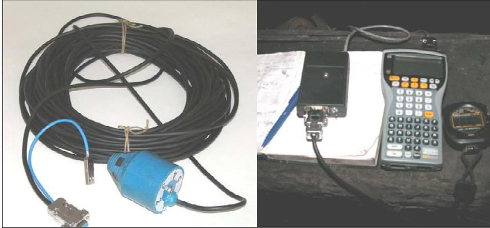
**Fig. 2** A gauges probe for long term measurement of stress tensor (left side), registration unit PSION (right side).
