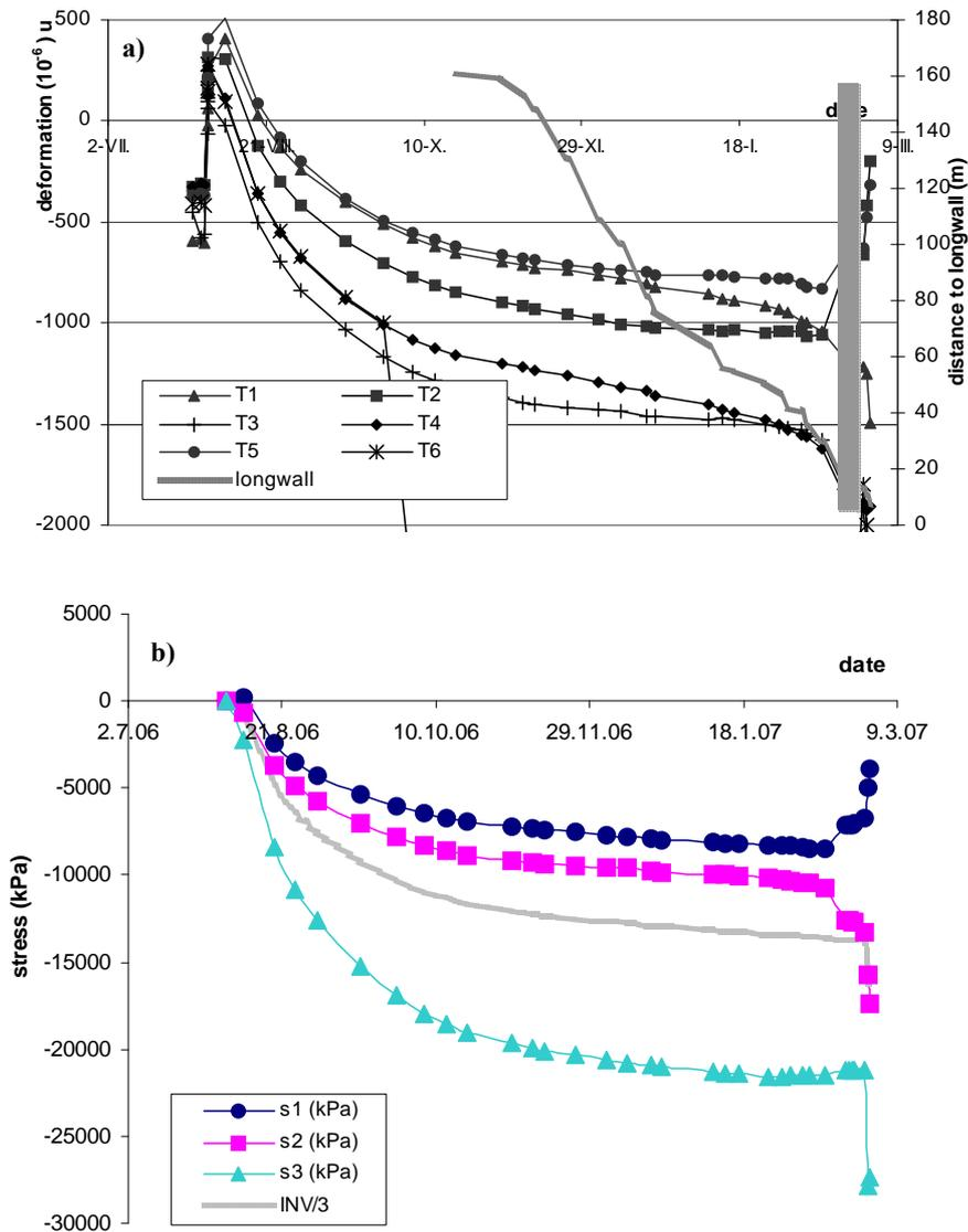
**Fig. 4** Probe 2<sub>6</sub>. a) record of deformation measurement on the gauges „T<sup>u</sup>“-type, b) calculated stress representation of the gauges deformations.
