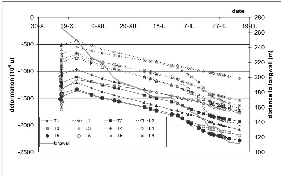
Fig. 6 Record of deformation measurement on the all gauges of the probe 3<sub>1</sub>.
