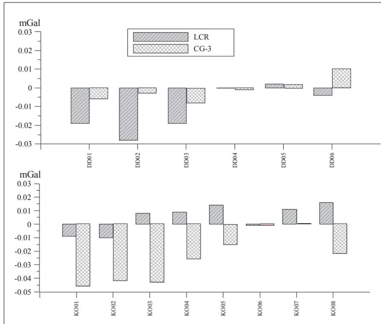
**Fig. 5.1** Time Temporal changes of the gravity field for profiles DD and KO in the time interval of 2005 – 2004.
