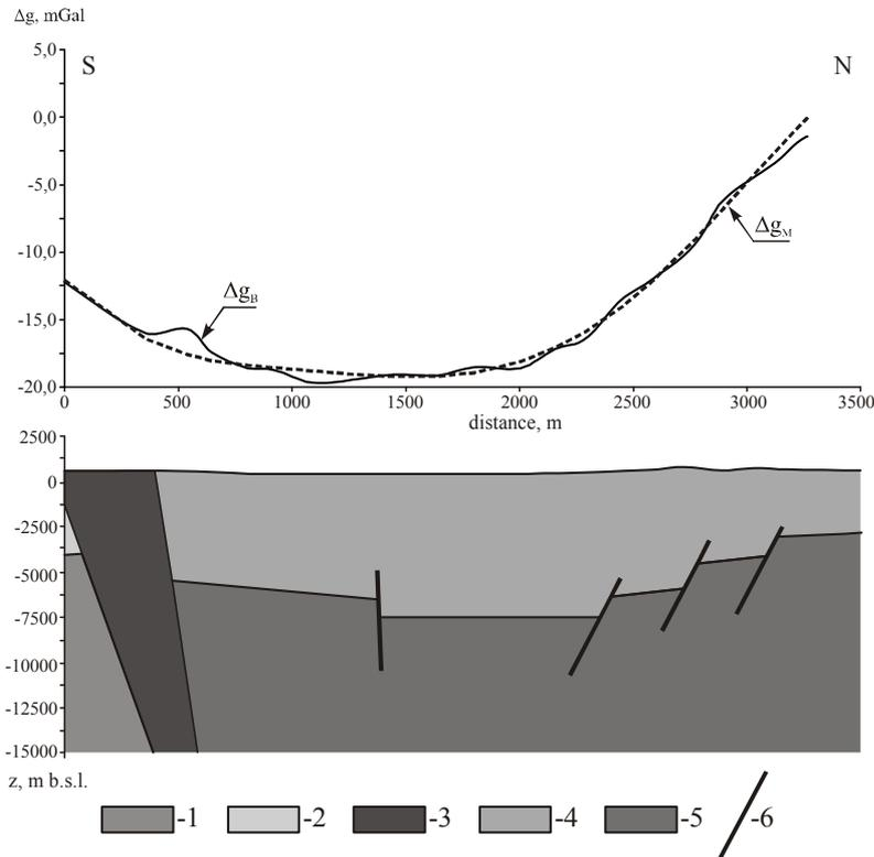
**Fig. 5.5** Results of gravimetric 2.5D modelling along profile DD. See Fig. 5.5 for explanation.
