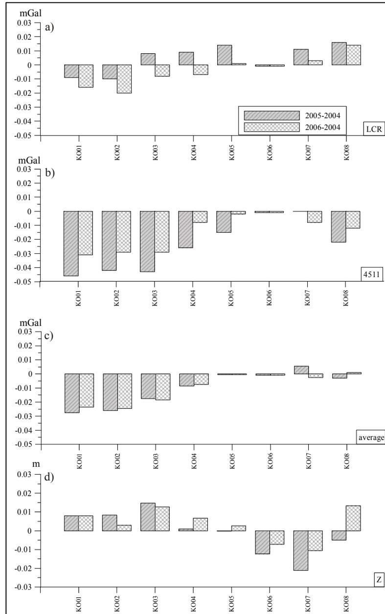
**Fig. 5.2** Temporal changes of the gravity and height at stations on the geodynamic profile KO for the time intervals of 2005 – 2004 and 2006 – 2004.
