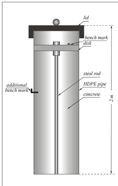
**Fig. 2.1** Scheme of a measuring point design.
