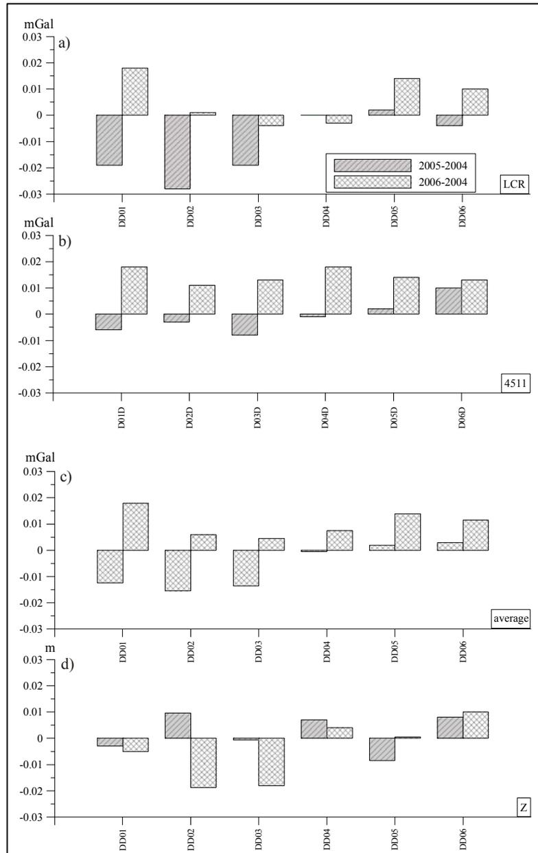
**Fig. 5.3** Temporal changes of the gravity and height at stations on the geodynamic profile DD for the time intervals of 2005 – 2004 and 2006 – 2004.
