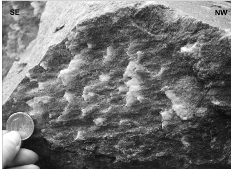
Fig. 2 Calcite slickenfibres on the NW-SE fault plane, limestone quarry near Vápenná village railway station.
