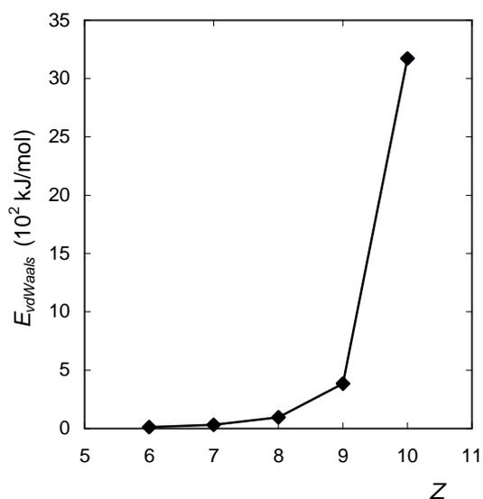
**Fig. 5** The dependence of the van der Waals energies (and consequently forces) in effect on the number of carbons in the cyclized molecules of meta n-alkylphenols (MM+ method, -CH<sub>3</sub> cyclization).
