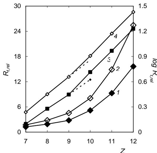
**Fig. 1** Non-linear dependence of the relative retention time ( $R_{t,rel}$ ) (lines 1 and 2) and divergence dependence of  $\log R_{t,rel}$  (lines 3 and 4) on the number of carbons in the molecule ( $z$ ) for the stationary phase of Apiezon K at a temperature of 130 °C in the case of n-alkylphenols. Full points – ortho n-alkylphenols, empty points – para n-alkylphenols. Similar dependences were found also in the case of n-alkylbenzenes. Based on Buryan and Macák, 1982, adjusted.
