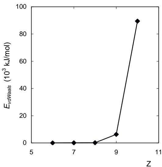
**Fig. 6** The dependence of the van der Waals energies (and consequently forces) in effect on the number of carbons in the cyclized molecules of para n-alkylphenols (AMBER method, -CH<sub>3</sub> cyclization).
