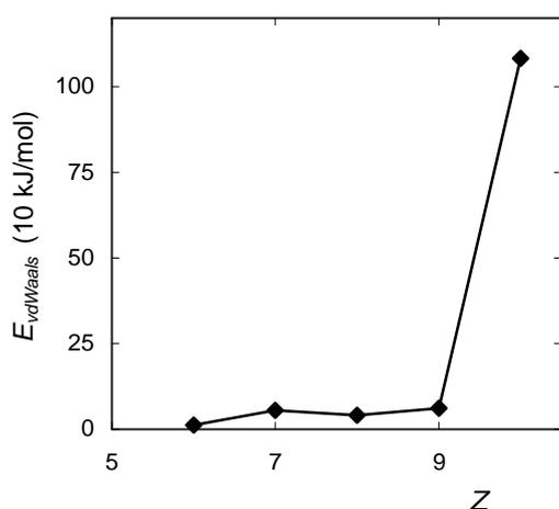
**Fig. 7** The dependence of the van der Waals forces in effect on the number of carbons in the molecules of n-alkylbenzenes cyclized into the position meta with respect to the substituent (the AMBER method, -CH<sub>3</sub> cyclization).
