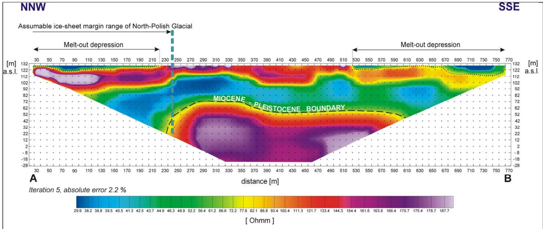
Fig. 4 Electrical resistivity cross-section along the Pilawa River valley.
