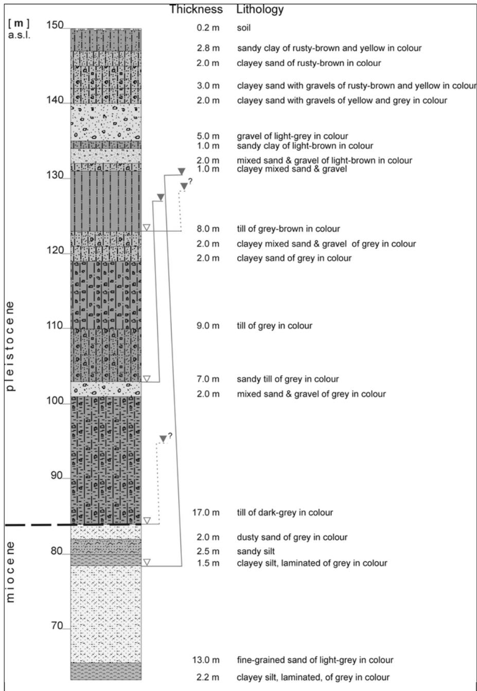
**Fig. 2** Geological profile of Liszkowo-PGR No 1638 bore-hole with piezometric levels of individual aquifers.
