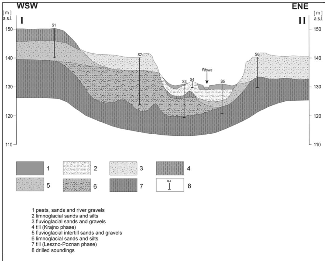
**Fig. 3** Pilawa River geological cross-section (Klimek and Lewandowski, 2002 modified).
