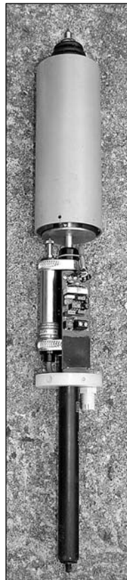
Fig. 10 Sensing part of convergence meter KK1.
