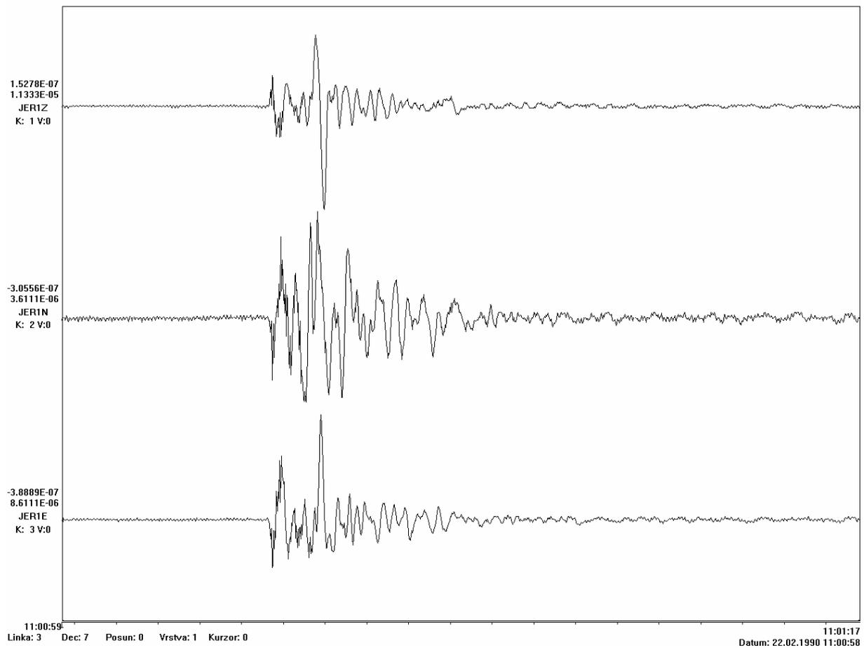
**Fig. 9** Example of wave pattern of blast generated in the quarry Krásno (recorded by station JER1).
