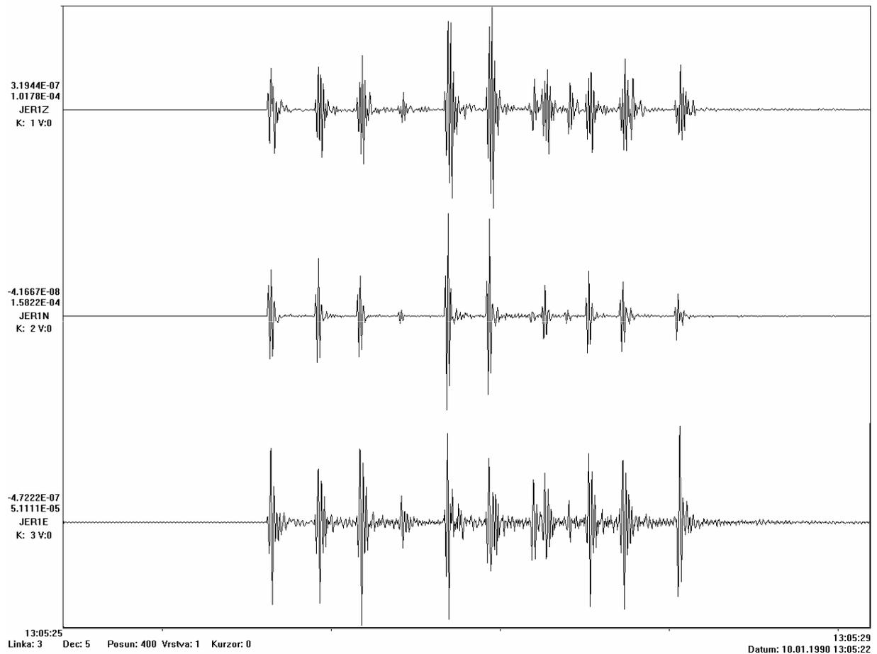
**Fig. 7** Example of wave pattern of a blast generated in the Jeroným adit (horizontal axis is local time, top down axis are vertical, N-S and E-W components).
