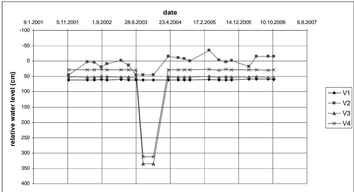
Fig. 5 Quarterly measurements of mine water fluctuation (locations V1 – V4).
