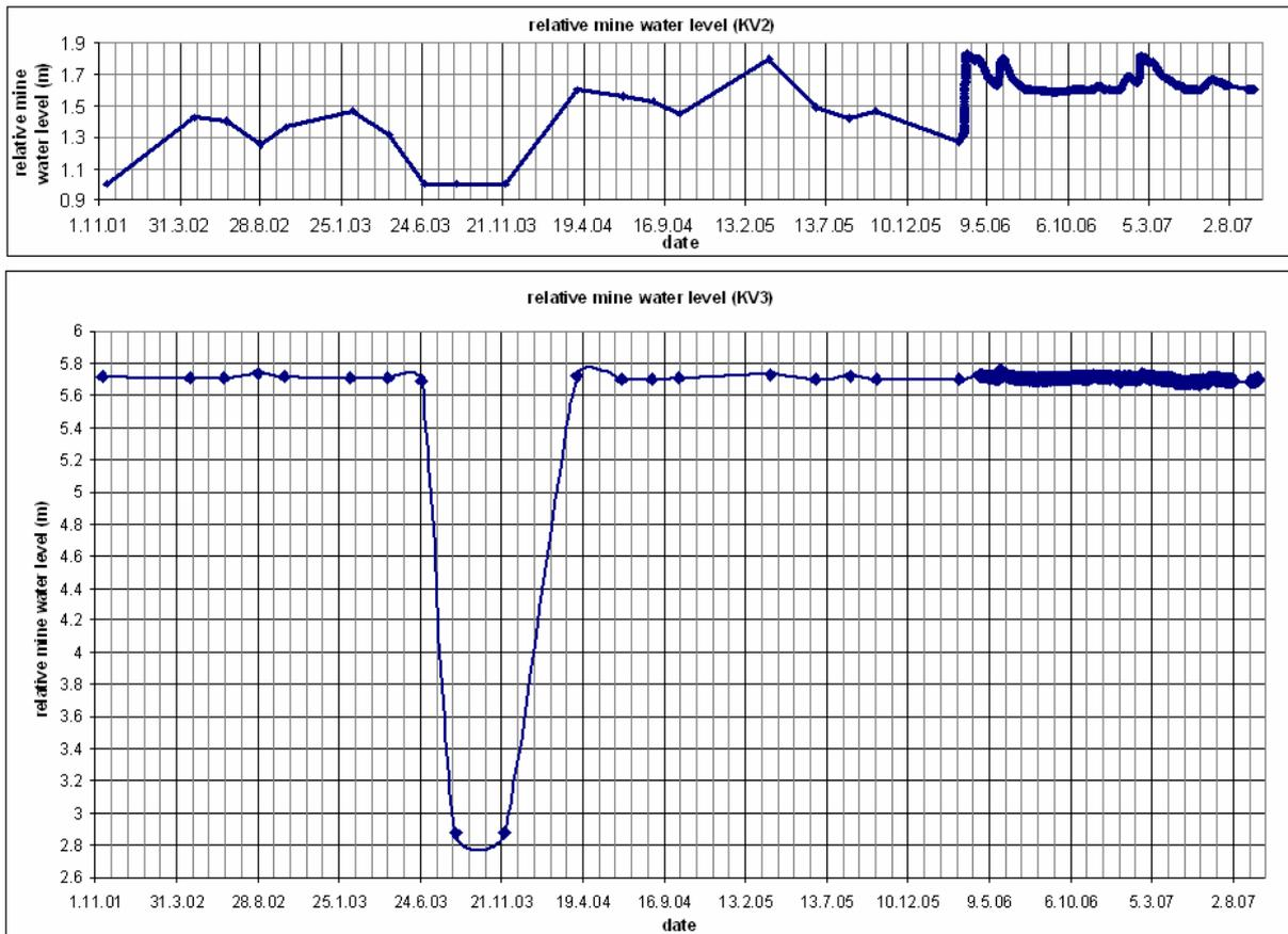
**Fig. 6** Fluctuation of mine water levels on locations KV2 and KV3 (quarterly and continuous monitoring).
