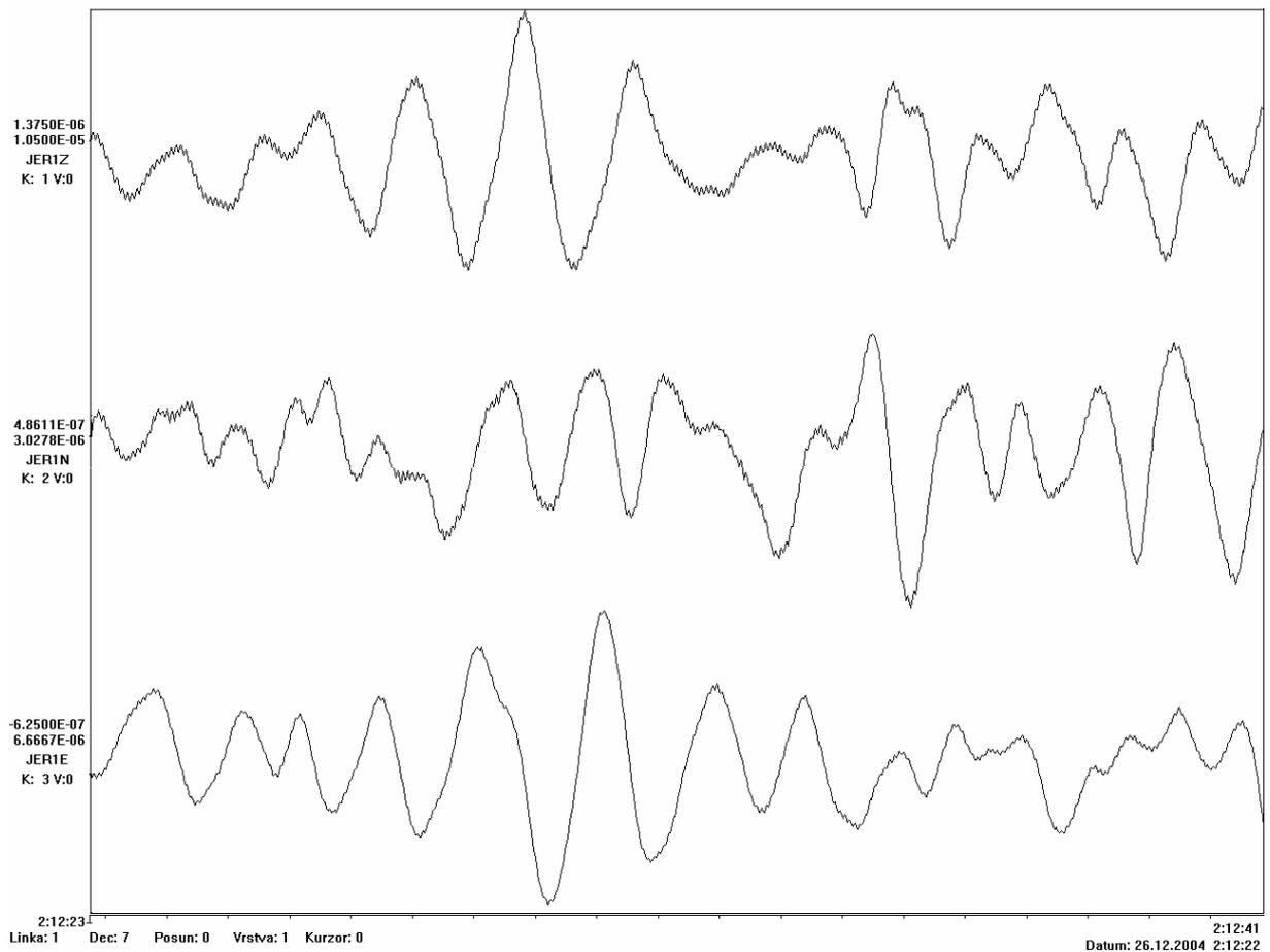
**Fig. 10** Example of distant earthquake record – non-identified part of earthquake from Indonesia.
