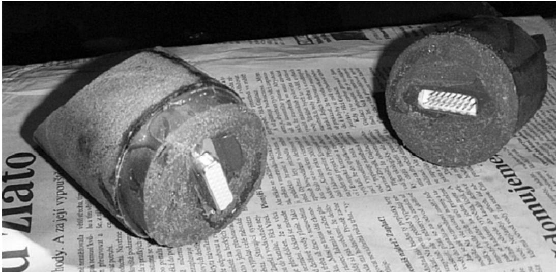
Fig. 8 The CCBO probe extracted from borehole after dissection in plane of separation.
