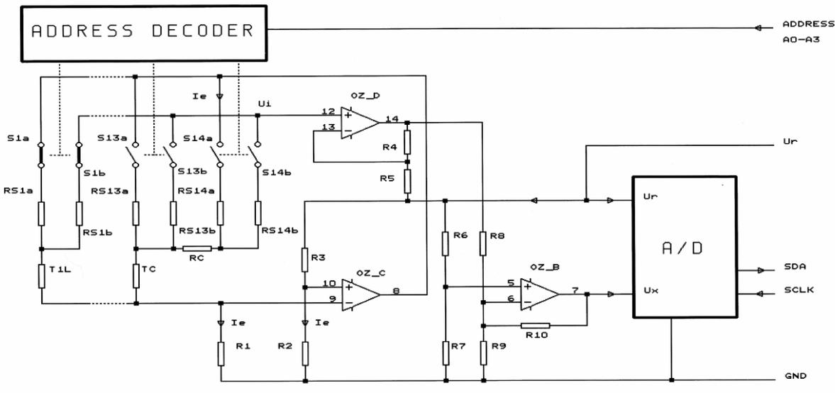
Fig. 4 Principal circuit diagram of multiplexed strain-gauge quarter bridge (MUX).
