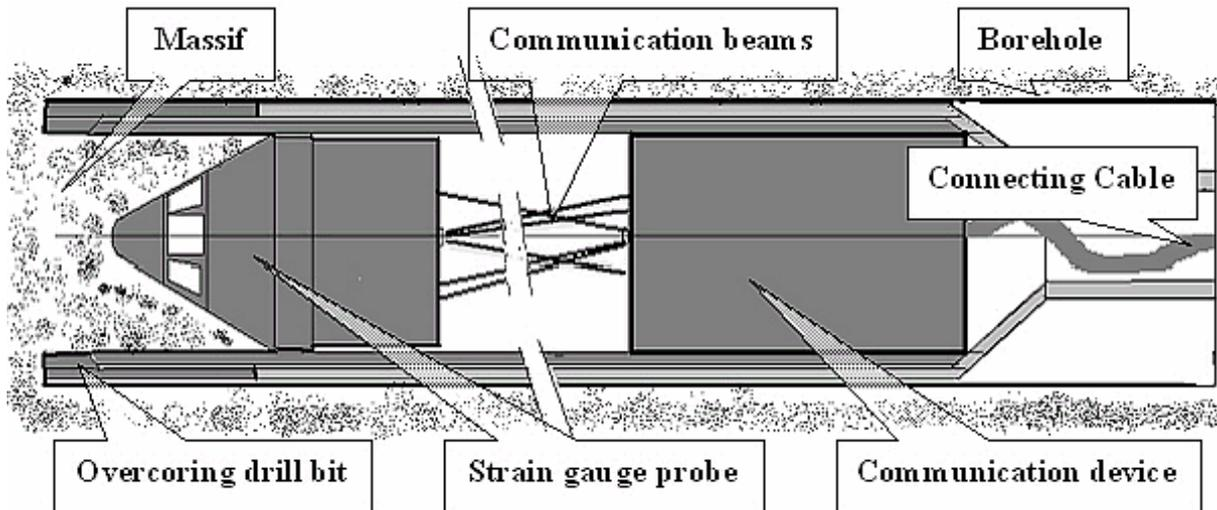
**Fig. 2** Conception of disposition of 1st generation CCBO equipment in borehole (Staš et al., 2005a).
