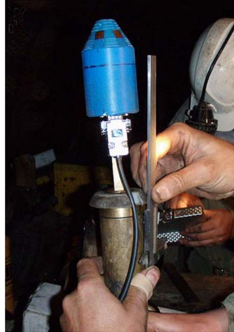
**Fig. 6** Preparing of CCBO installation to borehole. Separation plane is marked.
