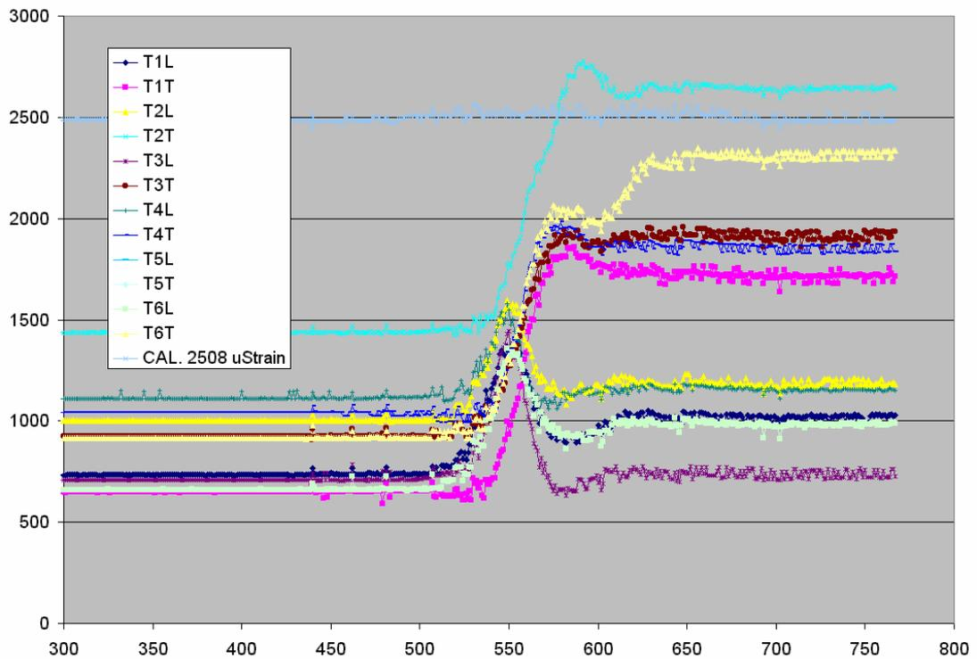
**Fig. 7** Plot of measured data. Over-coring experiment in Rožná Mine.
