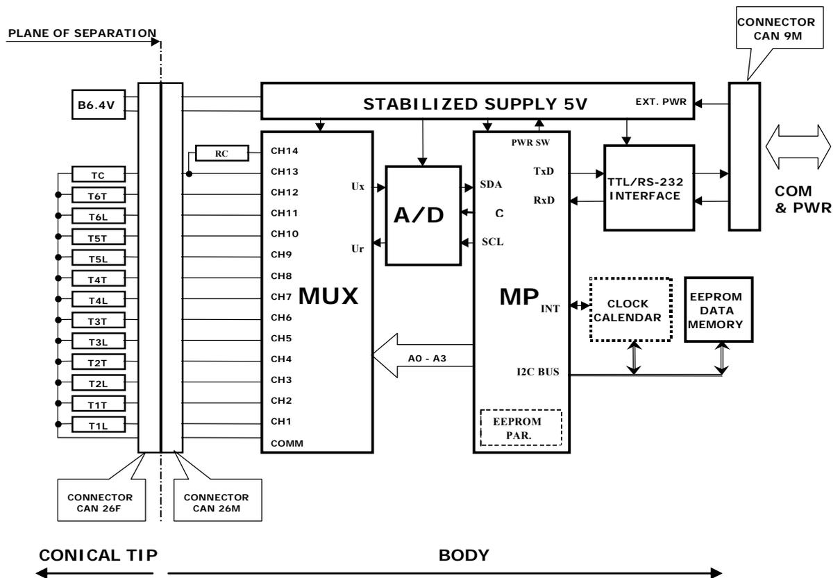
Fig. 3 Simplified block diagram of 2nd generation CCBO probe.
