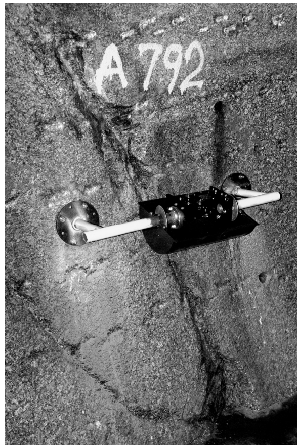
Photo 1 Gauge TM-71 installed across fracture of Krušné Hory Mts. orientation (120°/75°).
