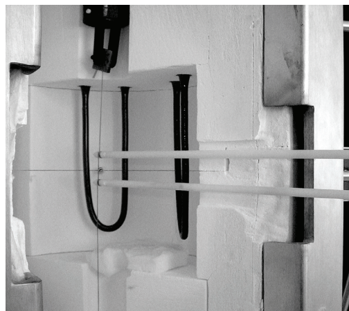
Fig. 1 View of alumina rods transducing the tow elongation to the extensometer through a slot in insulation of the furnace (now open).
