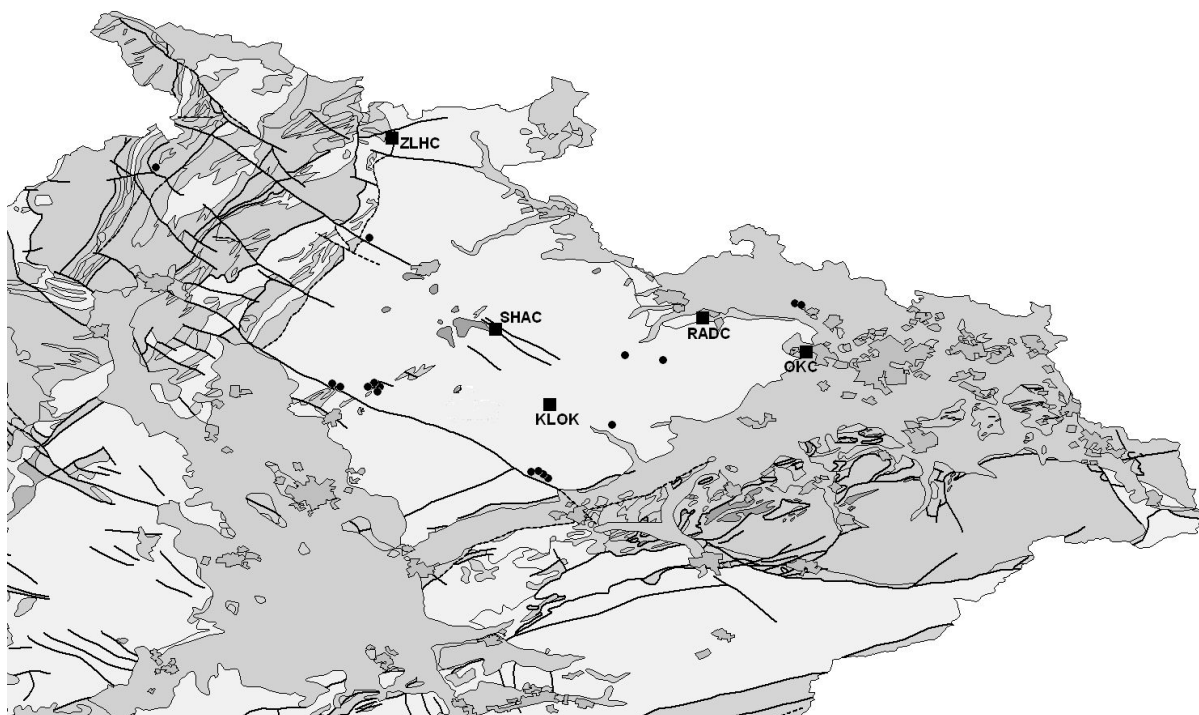
Fig. 1 A general survey of seismic stations (■) distribution and position of located epicentres (●).
