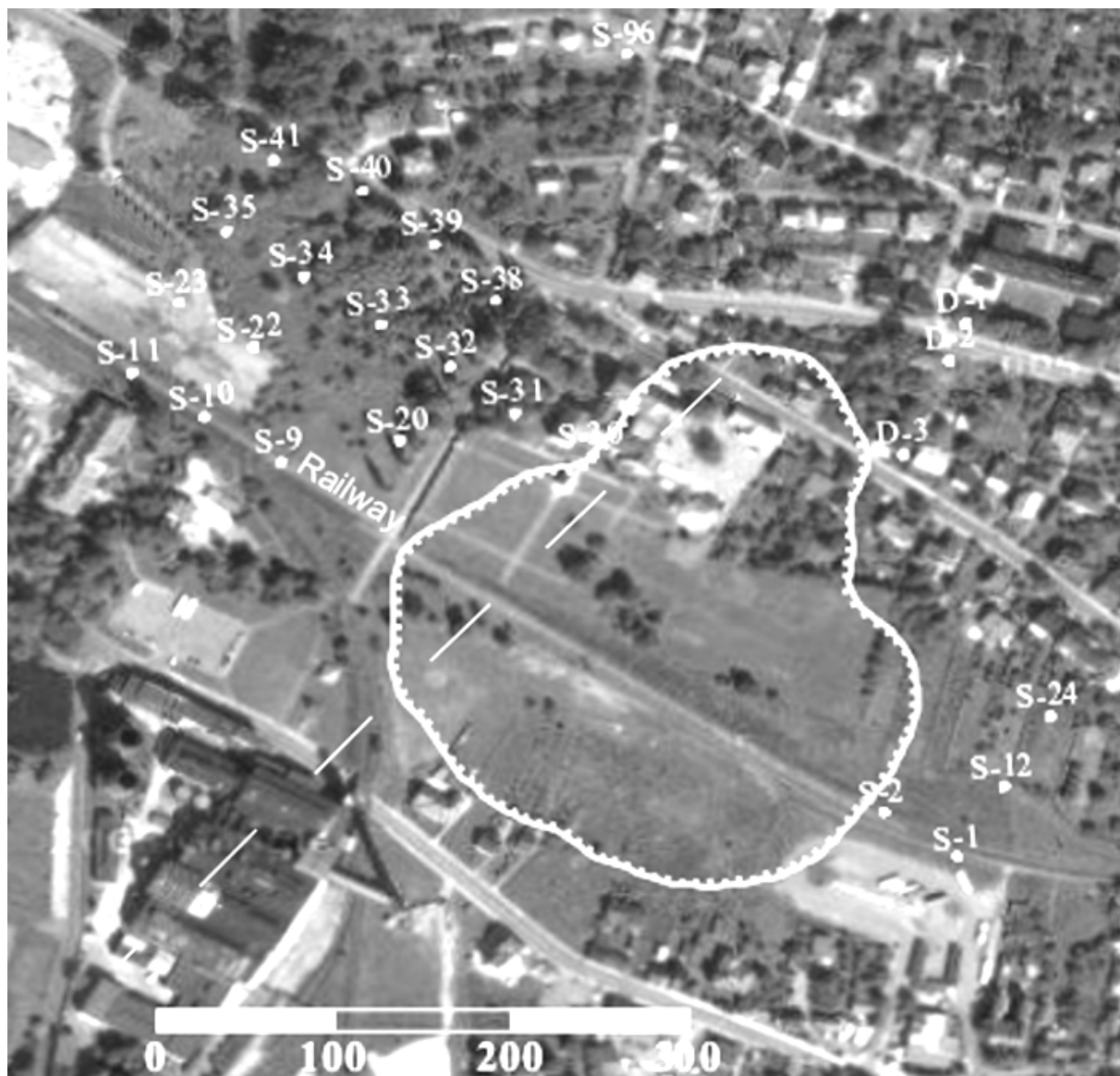
Fig. 1 The Serafa valley and the Cloister Hill in Wieliczka. Localization of surveyed benchmarks and a boundary of a subsidence bowl caused by water inflow into the Mina heading (white closed line). Dash line represents a localization of the cross section mentioned in the text.
